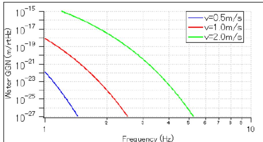
With this model, the water GGN limits the KAGRA sensitivity only if  $v$  exceeds  $\sim 10\text{m/s}$ .
