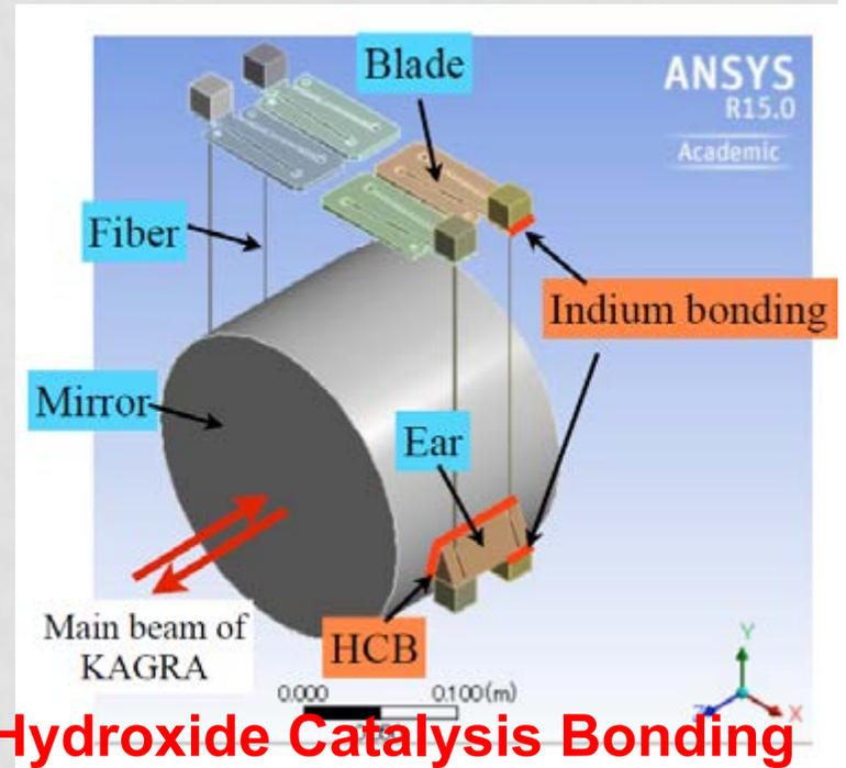
Hydroxide Catalysis Bonding
