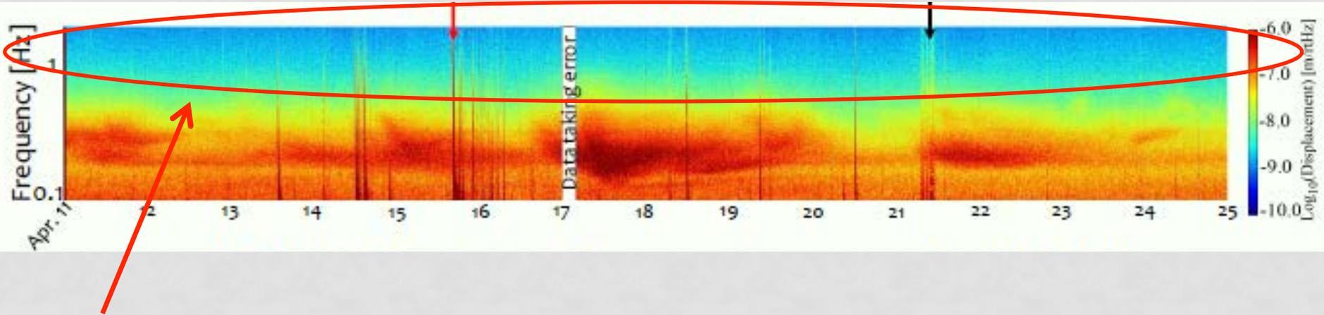
Around 1Hz, seismic motion is  $10^{-9}\text{m}/\text{rtHz}$  (**100 times smaller** than typical one) and almost **constant**. Requirement for control system should be modest.
