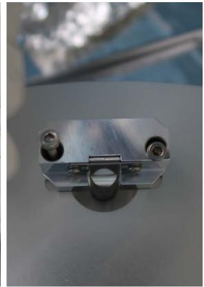
• For each prism, retract the translation stage, remove the prism holder and smear TBD amount of glue on the base of the prism.
