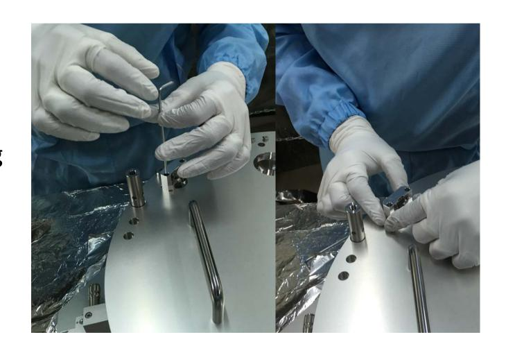
Remove the three screws holding the top plate, being extremely careful of the two near the flags.
