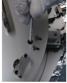
Test the flags with the magnet tester and place them near the optic at the corners where they will go: flags with N towards the tip at top left and bottom right, and flags with S toward the tip at bottom left and top right.
