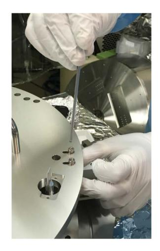
Retract the L-brackets (two visible screws and one in the hole). • Lift off the top plate, being extremely careful of the flags.
