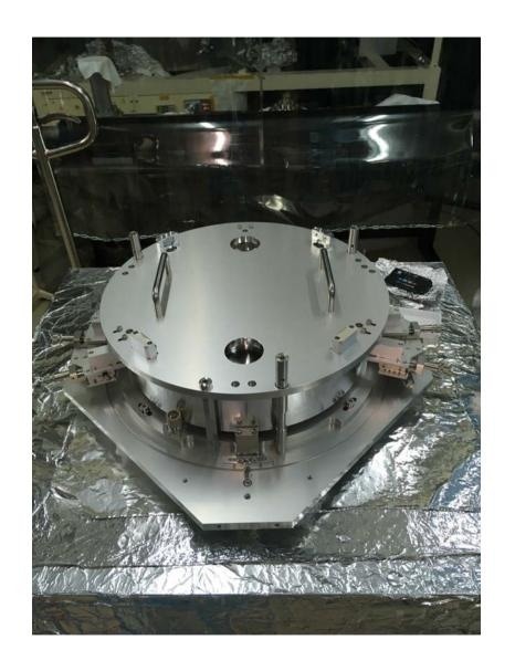
• Undo the lock screws on the translation stages for the primary prisms, and withdraw the stages till they are about 7 mm from the optic.
