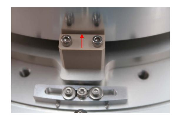
• Install two translation stage assemblies, big end to top, pressing each of them down and in against the three locating pins and secure with 3 M4 screws.
