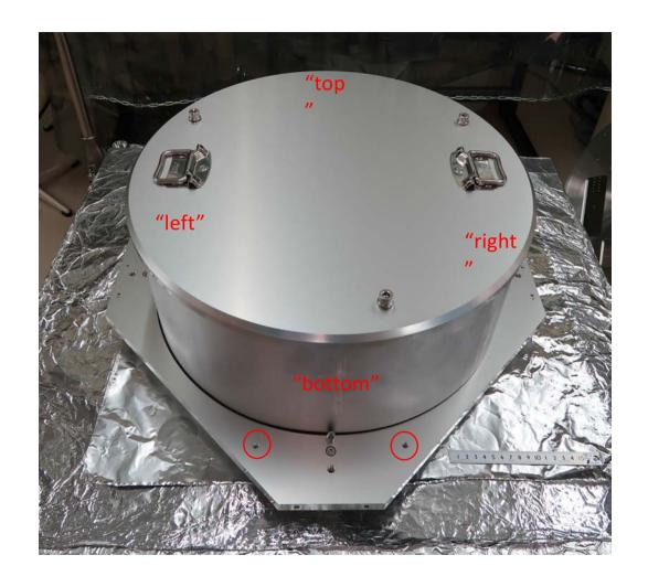
Remove the lid (three screws) and cylinder.
