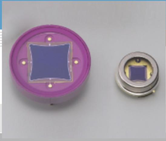
PSD (Position Sensitive Detector) is an optoelectronic position sensor utilizing photodiode surface resistance. Unlike discrete element detectors such as CCD, PSD provides continuous position data and features high position resolution and high-speed response.
