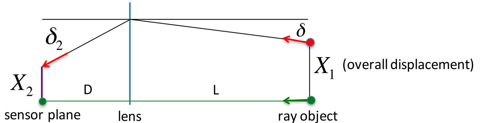
if the lens radius is  $R=2.5$  cm, the maximum measurable angle is  $\theta_{\max}=R/L= 19$  mrad yielding a spot displacement on the sensor of 3.8 mm
