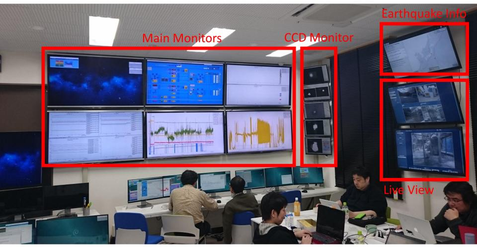
Main Monitor: You can check interferometer condition, temperature, humidity in KAGRA site. CCD Monitor: You can check output of CCD cameras. Earthquake Info (USGS website): You can monitor earthquakes around Japan. Live View: You can see live views in KAGRA site.
