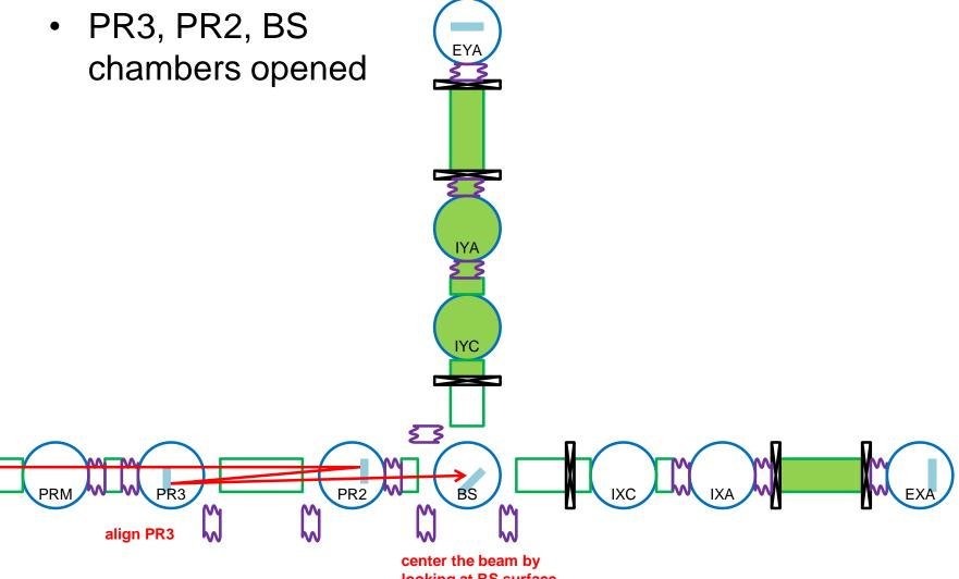
center the beam by looking at BS surface (beam radius 34mm)
