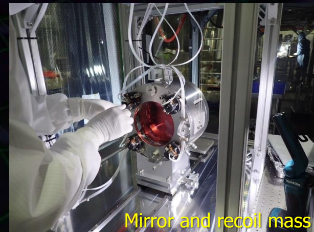
Hanging test for PR3 Type-Bp system (outside the tank) at Kamioka site.
