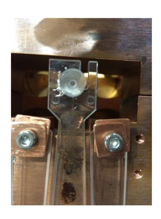
We tried to do the Indium welding, but the fiber head was not attached to the blade.
