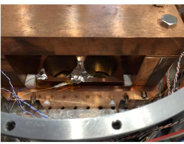
We inserted the Indium between the fiber head and the blade.
