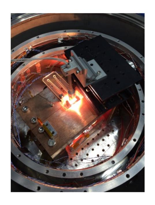
We tried to do the Indium welding between the blade and the sapphire block.
