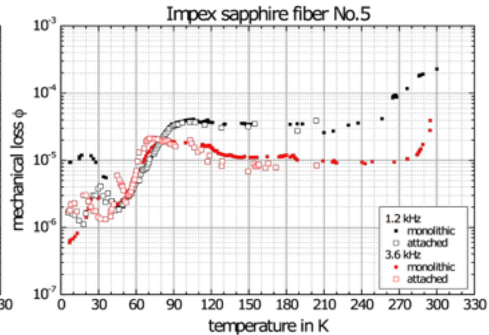
Comparison of two double nailhead fibers clamped at the monolithic (filled symbols) and the attached head (open symbols). At low temperatures it seems like the monolithic head provides lower losses.
