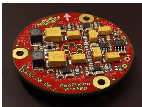
Figure 6.8: (Left) A picture of the geophone preamp. (Right) The conceptual circuit diagram of the primary amplification stage.
