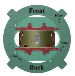
Attach the bottom plate ② JGW-D1504453-364 to the hexagonal pillars.
