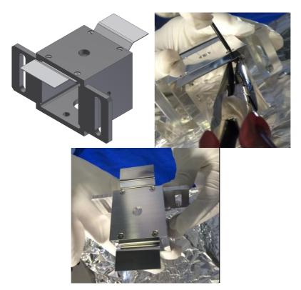
3. Fix the multipurpose assembly on top of the RM. Use the following screws:  $2\times ISO$  4762 M5×12mm coated.
