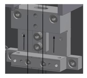
52. Fold the wires over the winch roller with the grooves and bring them to the roller with the clamp. Create tension by pulling the wires up, but not enough that would lift the RM. Make sure the wires go within the grooves of the two wire breakers around the RM. Fix the wires onto the roller with the clamps. Use the flat clamp in between the two rollers if necessary.
