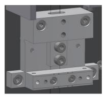
39. Remove the screws holding the back plate of the mirror box (the one with the handles) to the three horizontal hexagonal rods. The plate will not fall because there are four guiding rods holding it.
