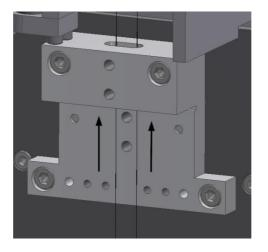
27. As in step 18, fold the wires over the winch roller. Before clamping them create tension by pulling them and making sure they go within the grooves of the four wire breakers around the TM. The figure shows one wire breaker and the grooves are clearly seen. Note that in reality the glass beads are not as neatly placed as depicted.
