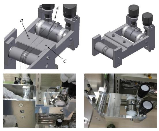
25. Create tension in the pair of wires by pulling them down from below the clamp assembly in the IM and then **softly** fix them with the upper clamp without the vertical grooves. Use 2 × ISO4762 M6 × 16mm coated screws.
