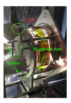
40. Remove the back plate by pulling from the handles.
