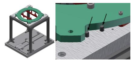
4. Clamp the ring to the frame at the four corners using the Misumi clamps. Use
