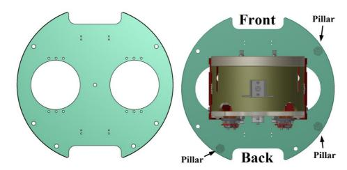
• Attach the 2 instances of the ① "Locking recoil mass" assembly onto the bottom plate JGW-D1504453-364. Use coated screws ① 12×ISO4762-M6x25mm.
