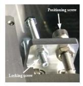
13. Release the locking screw and move the trolley away from the center of the table. Lock it on the far side of the table.
