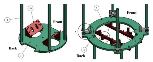
• The position where they should be depends on the particular optic which is being hanged. For PR2 and PR3 use the following configuration for the big ring JGW-D1504453-359 as seen from the top. Note that the plate is symmetric.
