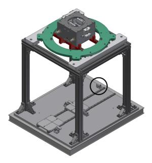
12. Align the Recoil Mass trolley the same way as the optic trolley in the previous step.
