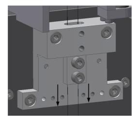
26. At the other side of the payload bring the other two ends of the wires up through the slit in the clamp all the way to the winches.
