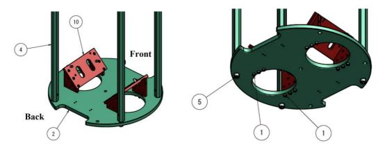
• Note that the stop set screws on the back side have to be higher than the set screws on the front side.
