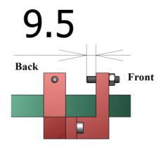
• Lateral studs (6): they should stick 7 mm toward the center. Adjust only the studs on the right side.
