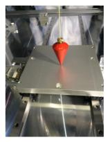
10. Slide the base of the mirror trolley under the IM and place its center where the plumb-bob indicates. Fix it in place with the positioning and locking screws on the sides. Use a nut to fix in place the positioning screw.
