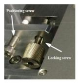
11. Release the locking screw and move away the trolley from the center of the table. Lock it on the far side of the table.
