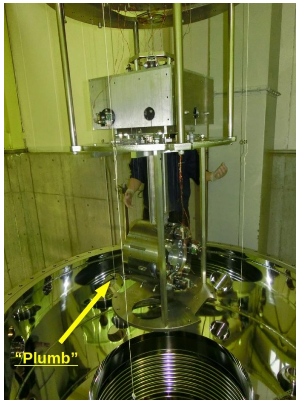
Fig.5: Plumbs as guides for suspension system installation
