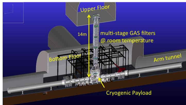
Figure 9 – Vibration isolation system with cryogenic payload.
