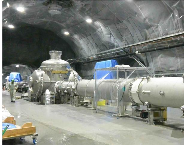
Figure 11 – Cryostat for cryogenic payload and cryogenic thermal radiation shield pipe at Y-front room.
