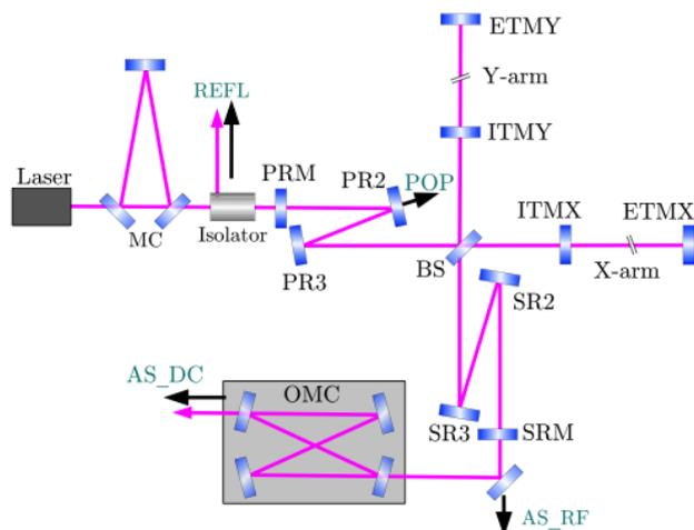
Figure 4 – KAGRA interferometer design. This is dual recycled Fabry-Perot Michelson interferometer configuration with input and output mode cleaners<sup>15</sup>.
