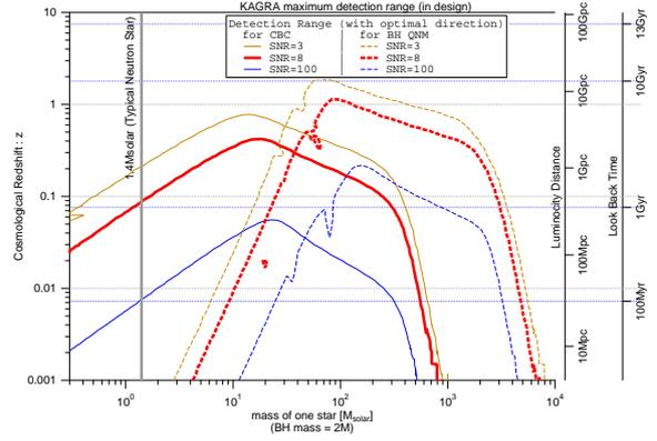
Figure 3 – Detectable range of GW signals from Neutron star binary coalescence (solid lines) and quasi-normal mode of black hole (dashed lines)<sup>13</sup>.
