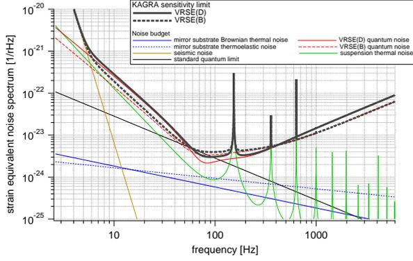
Figure 2 – Design Sensitivities of KAGRA. The thick black solid-line and the thick black dashed-line show the total sensitivities in detuned and broadband mode in interferometer, respectively. Green and blue lines show designed levels of thermal noises, and thin black line shows standard quantum limit.
