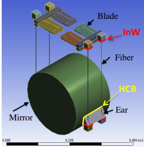
Figure 6 – Sapphire suspension system. HCB: hydro-catalysis bonding. InW: indium welding. HCB is used to contact between two ears and mirror substrate. And InW is used as replaceable contact among blocks at both end of fibers, blades and ears.
