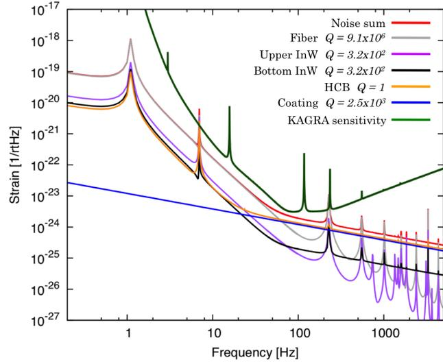
Figure 7 – Estimated thermal noise components with sapphire contacts and coating. Mechanical  $Q$  of 1.0 for HCB, 320 for indium welding, 2500 for coating and  $9.1 \times 10^6$  for fiber are assumed here<sup>20</sup>.
