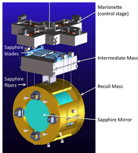
Figure 8 – Mechanical design of cryogenic payload
