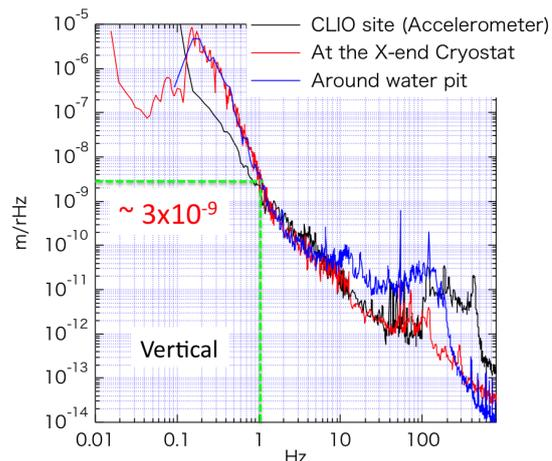
Figure 5 – Measurement result of vertical seismic vibration around main-mirror cryostat in X-end room (red line). Blue line shows vertical seismic vibration level in front of water pit. Both data were measured by a seismometer, Guralp CMG-3T, which has no sensitivity over 200 Hz. Black line shows vertical seismic vibration measured in CLIO site, where is in same Mt. Ikenoyama, by laser accelerometer, which has no sensitivity below 0.1 Hz.
