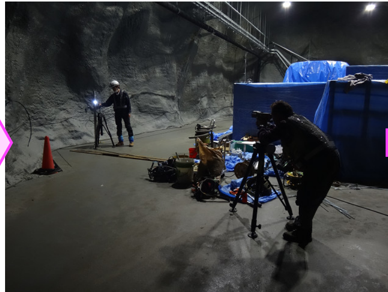
Reference pole(s) set and surveyed by KEK
