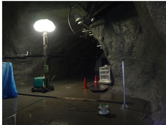
We also put height level standard bars w/ optical and LT targets.
