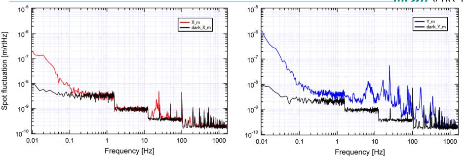
limited by digitization noise Thermal drift is seen below 0.1 Hz worse than X direction
