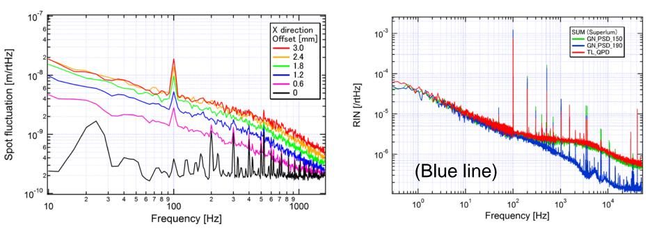
Consistent with RIN measurement within difference factor of 2 (The left response has two times smaller RIN than the right graph shows) => an individual difference of SLD
