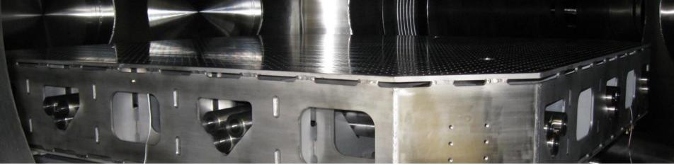
Transfer function —— Horizontal isolation performance: -80 dB at 4 Hz
