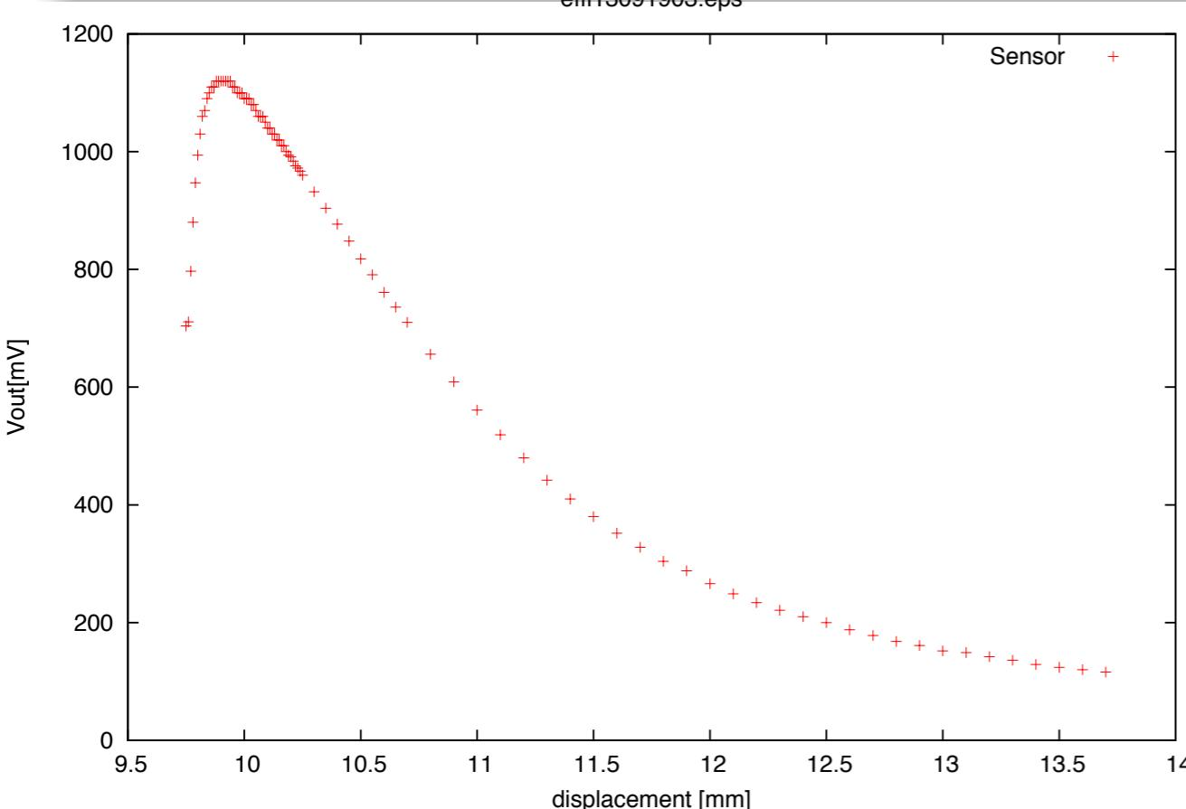
This is a reflective type transducer based upon detecting the intensity of reflected light.
