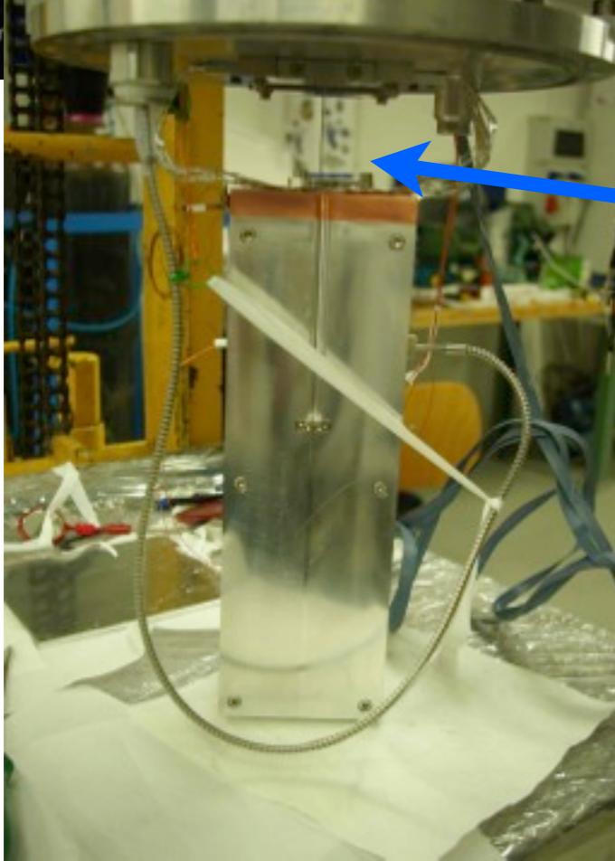
Double pendulum (3 wires)
