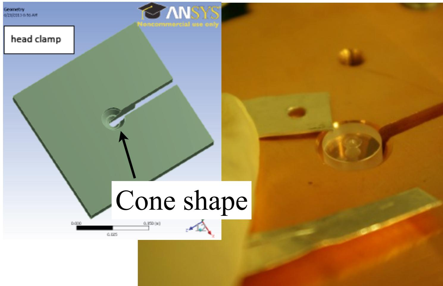
The fiber is fixed with stainless plate and cone shape copper holder.
