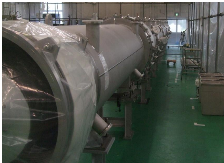
Radiation shield tube (17m) is under test
