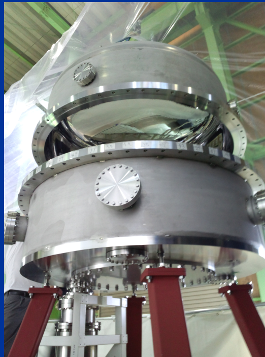
Seal test of the top-chamber
