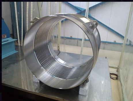
Bellows for each duct
