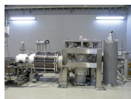
Pic1: Cryocooler Unit
