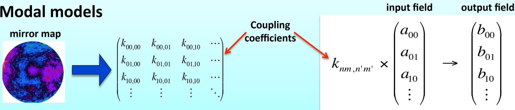
Matrix of coupling coefficients calculated from the mirror map transform the input field described by HG amplitudes into the output field described by HG amplitudes.
