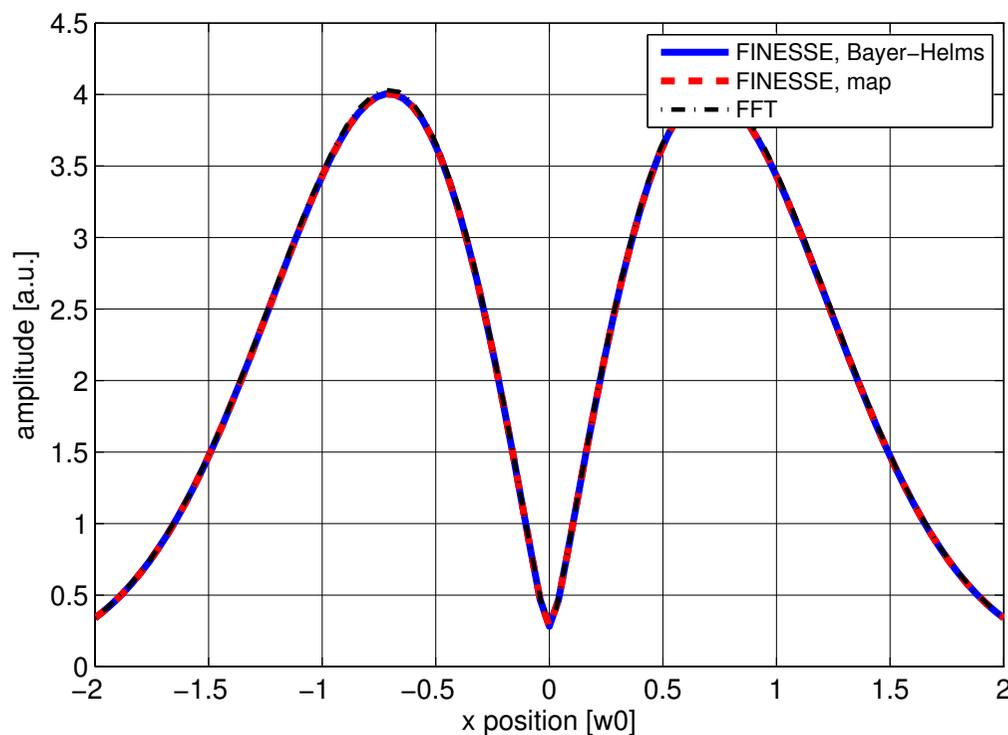
Reflected field with HG00 component removed, cross-section
