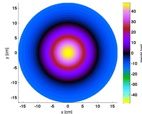
ETM thermal map with curvature removed
