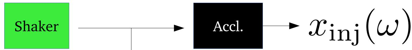
$$T_i(\omega) = \frac{h_{\text{inj}}(\omega)}{x_{\text{inj}}(\omega)}$$
