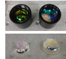
Different collimator lenses made of BK7.
