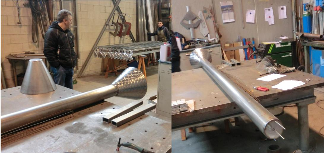
At the closed end, two 6 mm tubes allow the insertion of the type-K thermocouple for feedback, and of the purge Argon gas. The purge gas flows through the pipe and leaks through the two cones of the access port.
