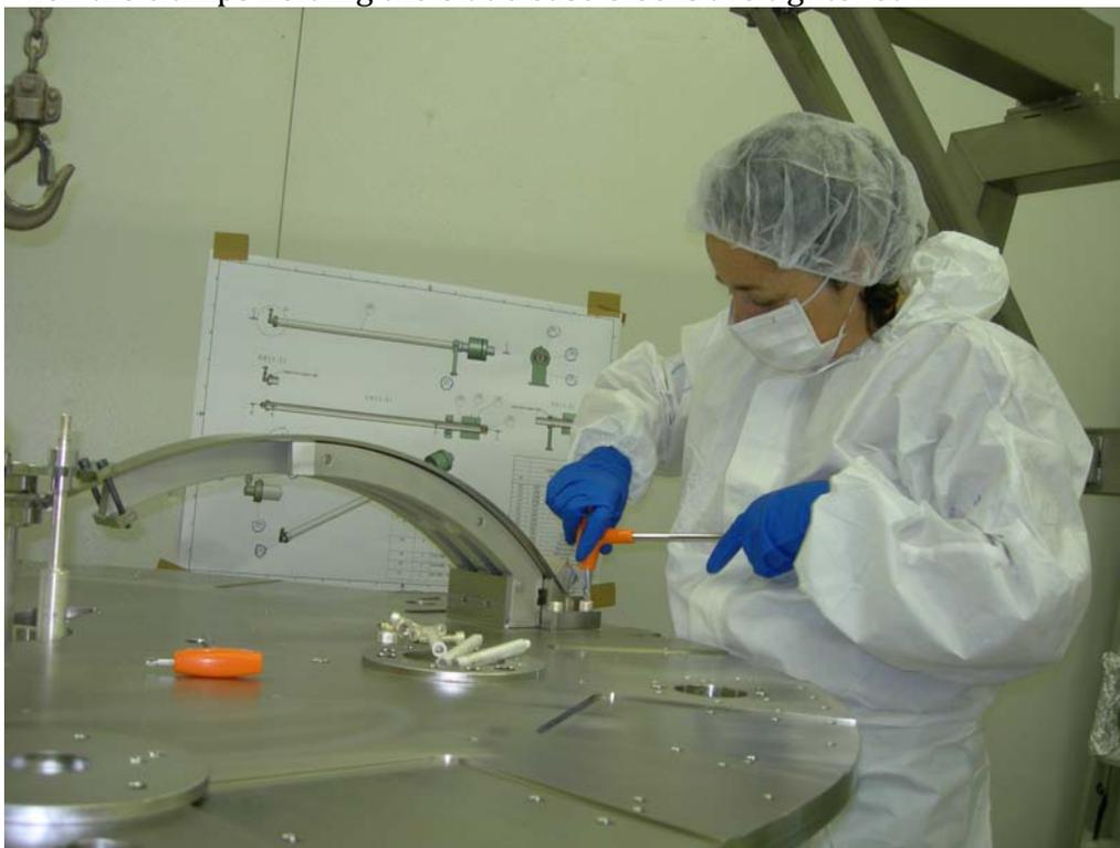
To release the pre-stressed blades the holding screws are lubricated with ultrapure alcohol
