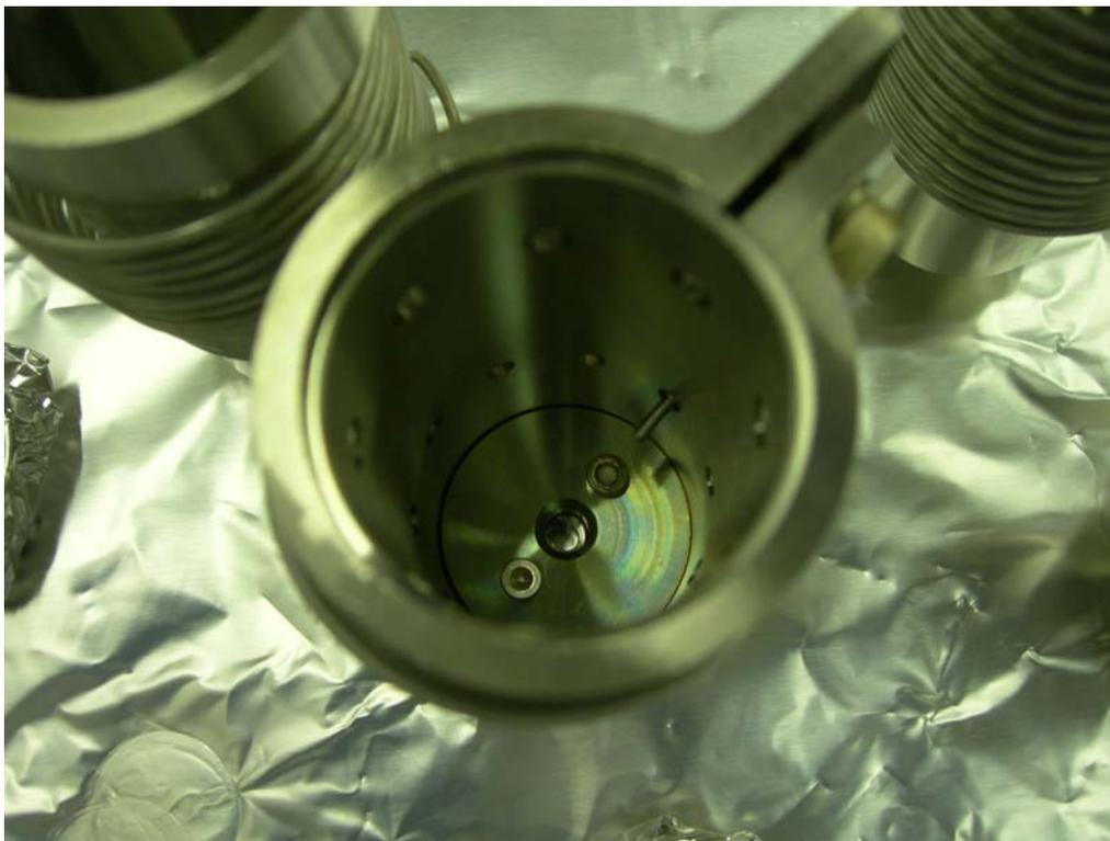
The flag cap can be easily oriented on the cap by means of two screwdrivers, one through holes designed for this purpose, and one in the locking mechanism slot.
