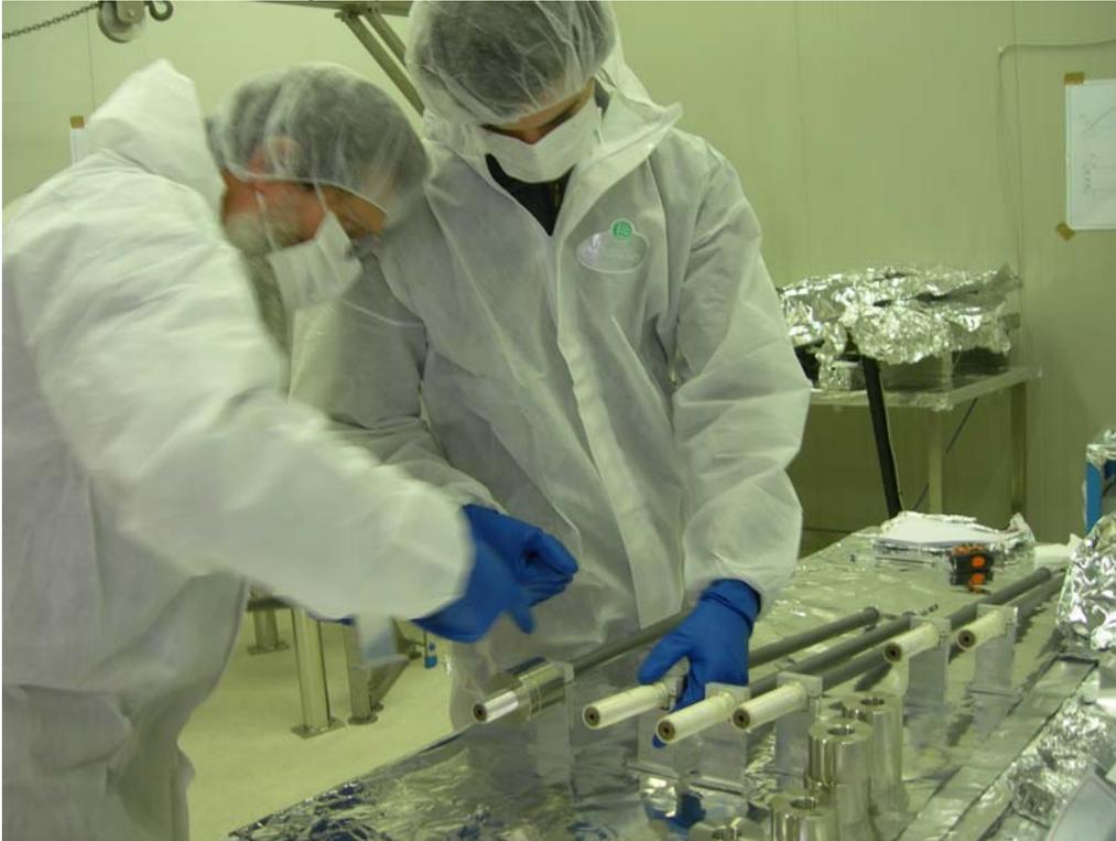
For assembly and transport the counterweights are mounted all the way in. In this configuration the magic wand is neutral and would have no effect. When installed, the counterweights will be moved backward by a pre-determined amount to generate the percussion point cancellation effect.
