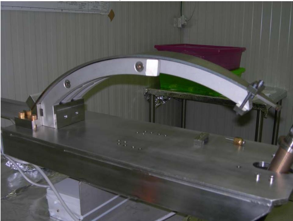
the block is unbolted from the tool and the pre-stressed blade is ready for assembly in the filter.
