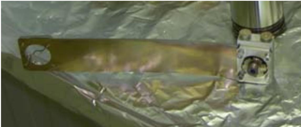
The mounting of the nut and the anti rotational blade are tested on the filter, then disassembled.
