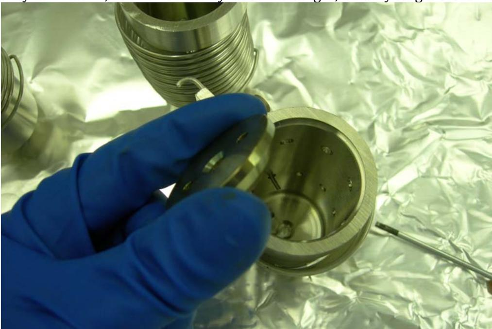
The safety ring bolts at the bottom of the cup, after the suspension wire is in place. It will allow the vertical motion and rotation of the wire without allowing it to misalign laterally. The flag cap and its radial screw locking mechanism is visible as well
