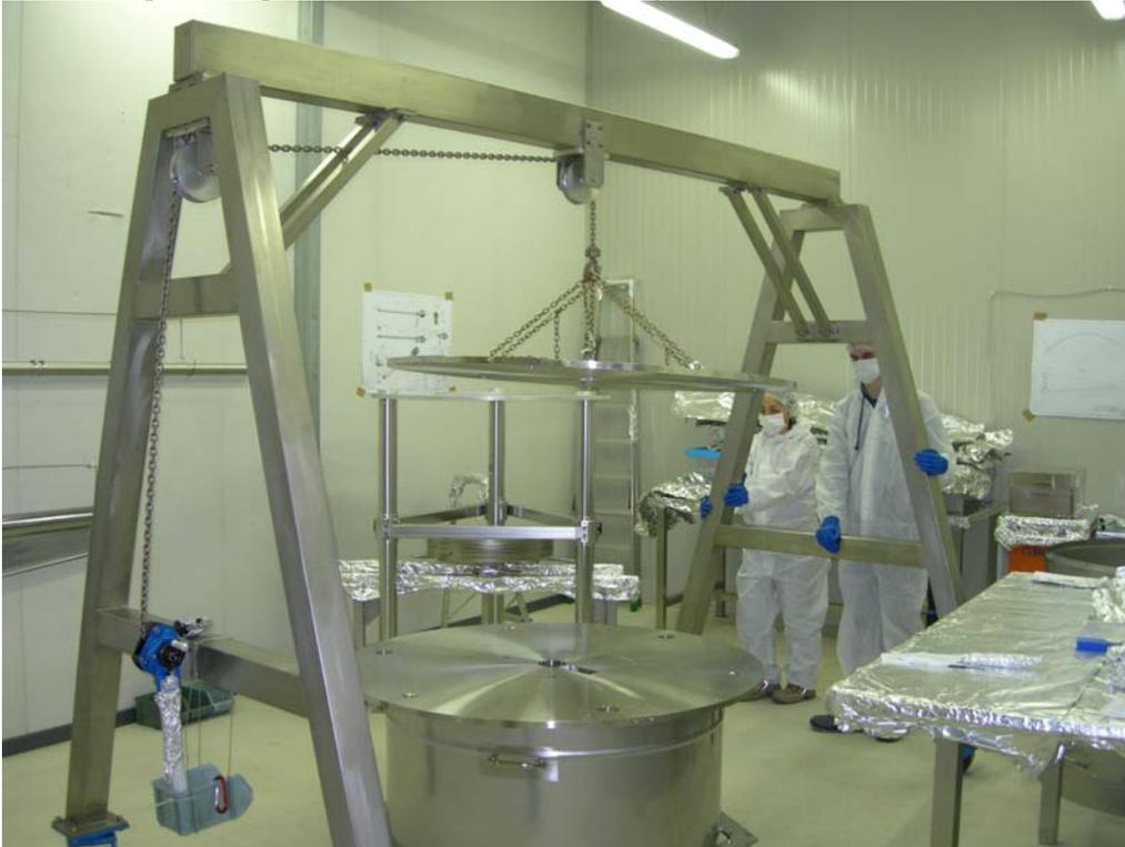
The keystone holding tool is fastened below the base plate.
