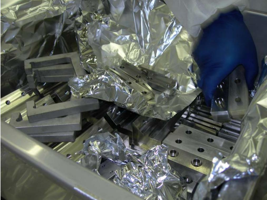
The canisters are then lowered in the oven for air bake at 200°C for 24 hours.
