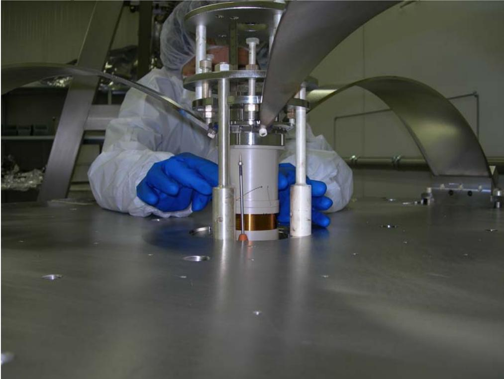
The LVDT primary and actuator wires are brought up to the top surface of the base plate.
