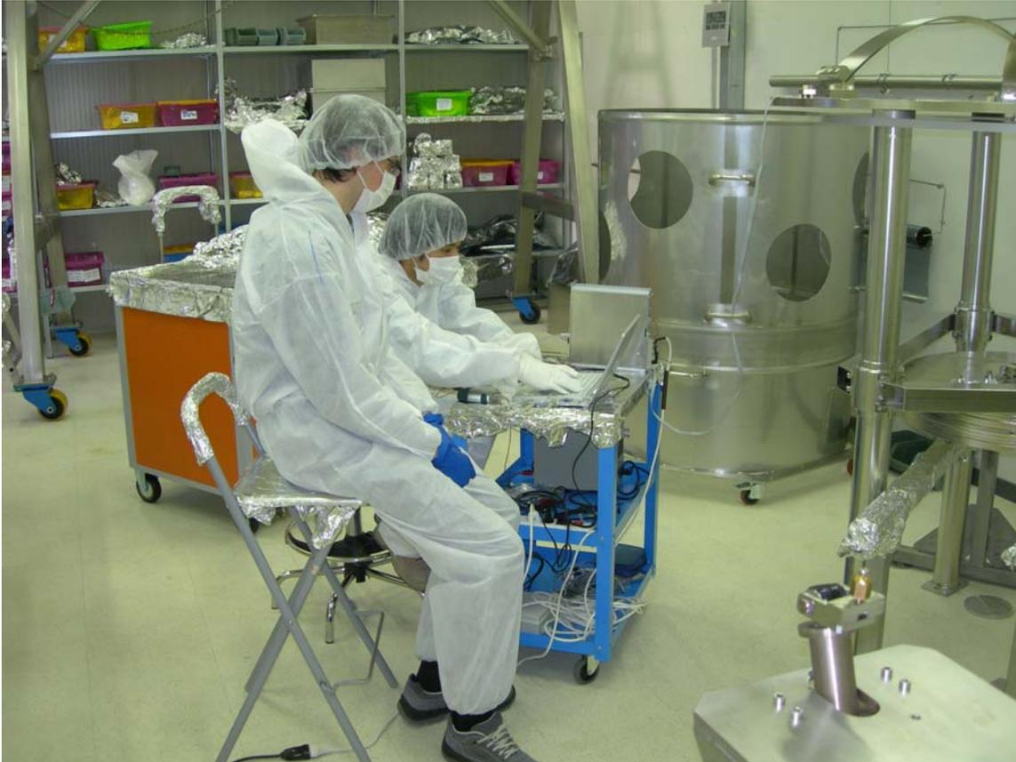
The radial compression of the filter is changed by incremental steps, thus changing its resonant frequency. At each step the optimal working point of the filter is found, by changing load weights and, at low frequency, by help of the filter hysteresis (see separate report by Paolo and Takanori). Finally the filter oscillation is excited and recorded to study the filter's behavior.
