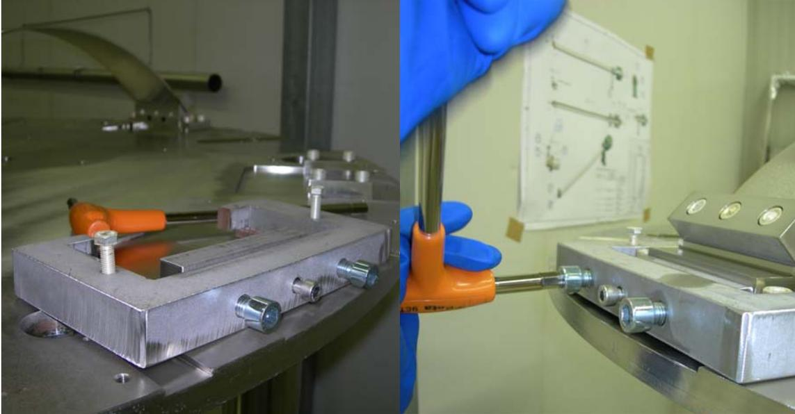
The radial compression is performed symmetrically and progressively on all three blades.
