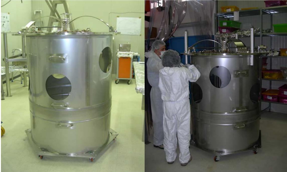
In order to keep the filter clean, it is not lifted directly by the crane, which may drip dirt. Instead the Oven cap is used as an intermediate dust and grease shield.
