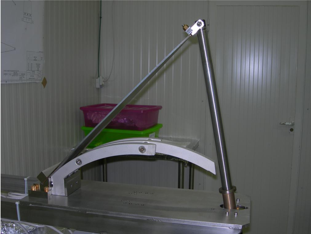
The actuator head can swivel and has a slot that accepts the blade's nose. A safety cap entraps the nose in the actuator head and is held by a screw passing through the hole in the blade's nose.
