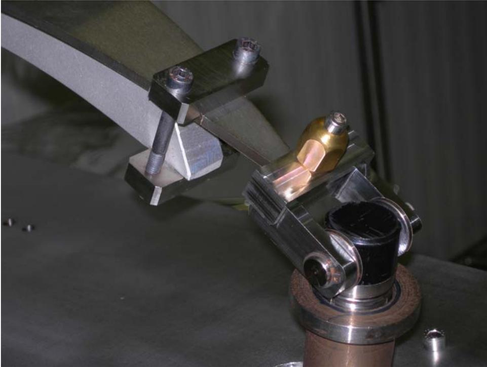
The actuator is disconnected, from the blade
