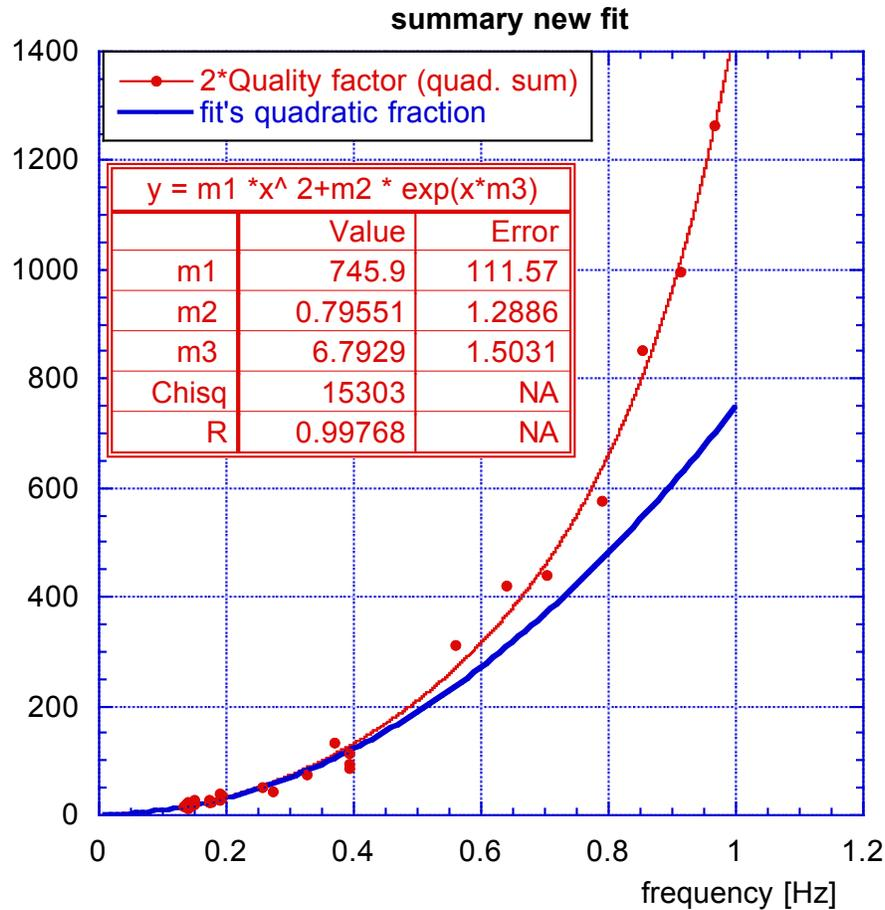
Comparing with the GAS spring tested in R. DeSalvo, et al., figure 30, the quality factors are higher, while the exponential departure point from the quadratic curve happens at 0.4 Hz instead of 0.2 Hz
