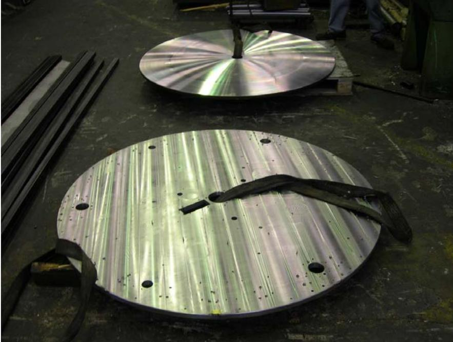
After machining, cleaning and etching, the base-plates were further baked 24 hours at 200°C to induce all possible warping before assembly, and for UHV cleanliness.
