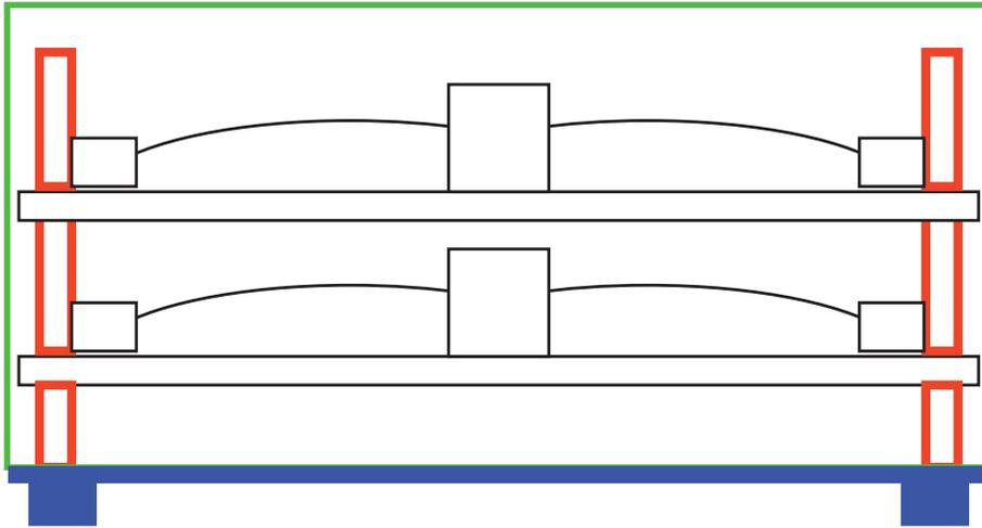
When a second filter is ready it is moved in, wrapped in aluminum foil and lowered on the waiting spacers of the lower filter in the crate.
