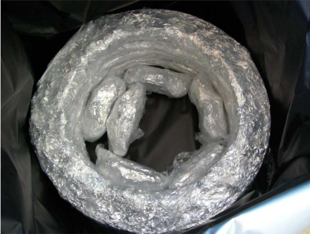
Water absorbing packs are added before welding the water barrier bag closed
