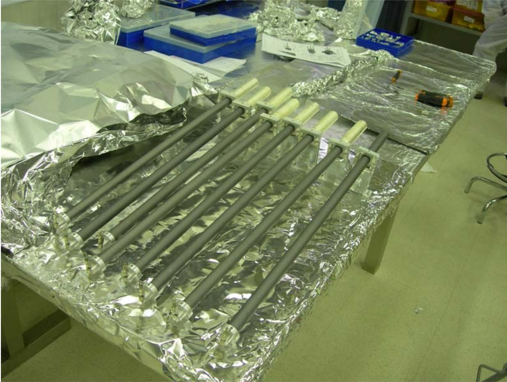
Finally the counterweight, formed by two cylinders, is screwed on the threaded insert.
