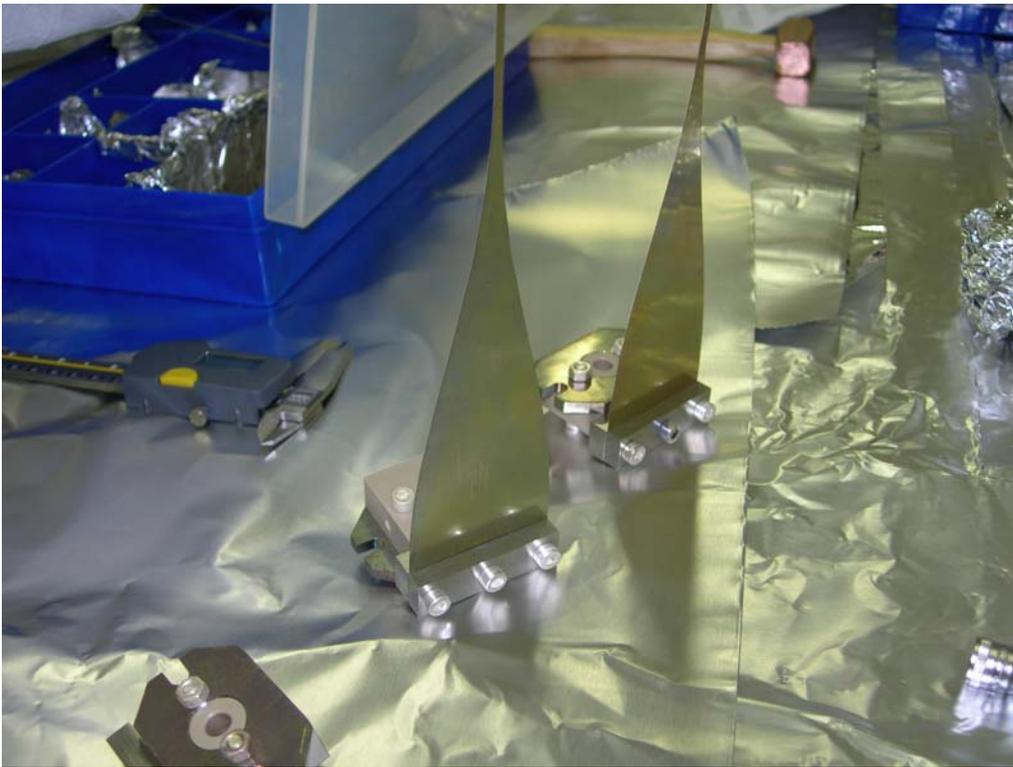
The anti-rotational rod is forced in the flange supporting the motor. Two anti-rotational rods are foreseen, but only one is mounted, because it may be sufficient and two rods may render the movement harder. The second rod is packaged together.
