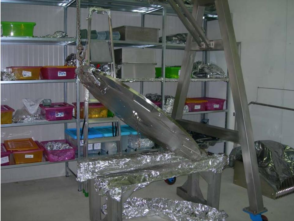
The base plate is then lifted from the inspection bench and moved to the assembly and testing tower
