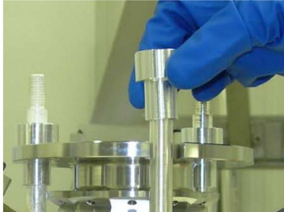
and the keystone end-stop plate is mounted and locked in place, and the columns supporting the rotational mechanism's plate are added.
