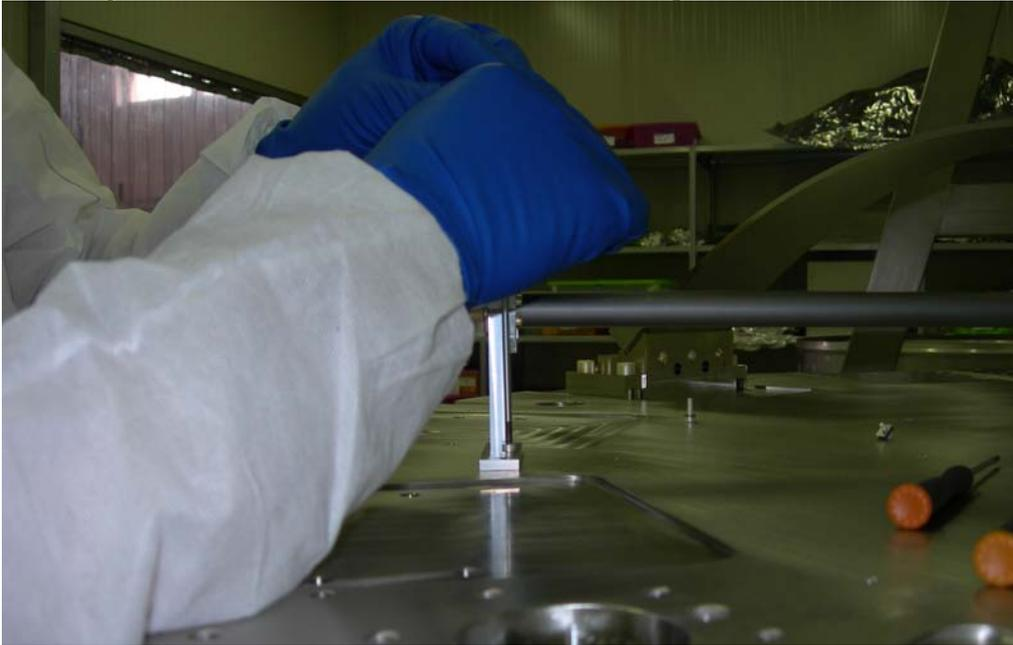
Before locking the wand's foot to the base plate, the alignment of the tip hinge must be checked for verticality.
