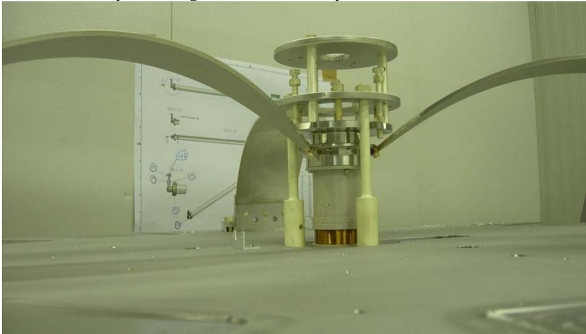
A 1 m long threaded rod is attached inside the keystone, and loaded with slotted load disks of various weights, until the filter starts floating and the upper end-stop screws can be retracted. Suitable safety stands below the disks insure against accidents.
