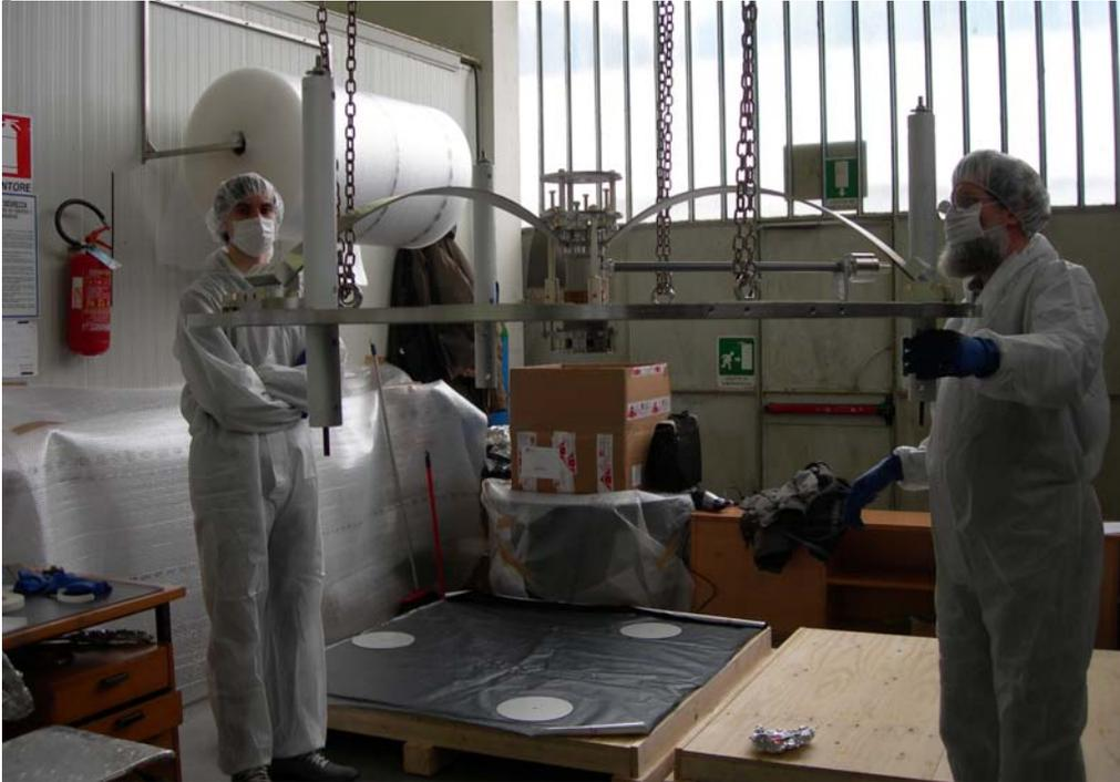
The filter is wrapped in UHV compatible aluminum sheet
