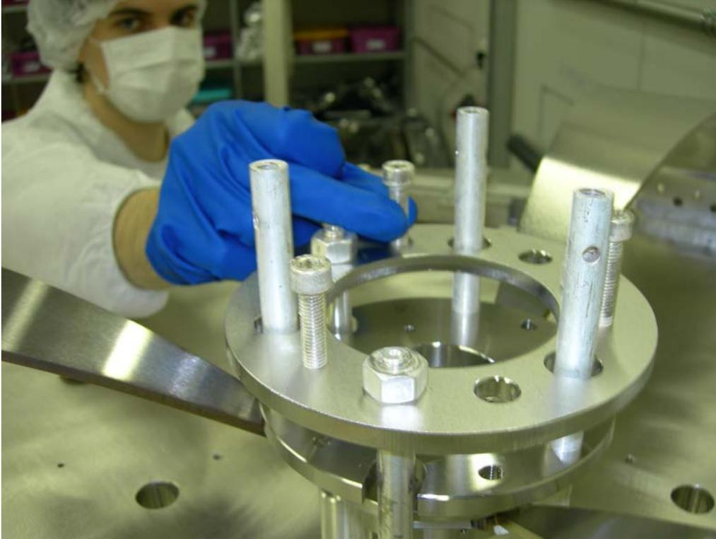
The rotation mechanism plate is mounted on its columns and locked
