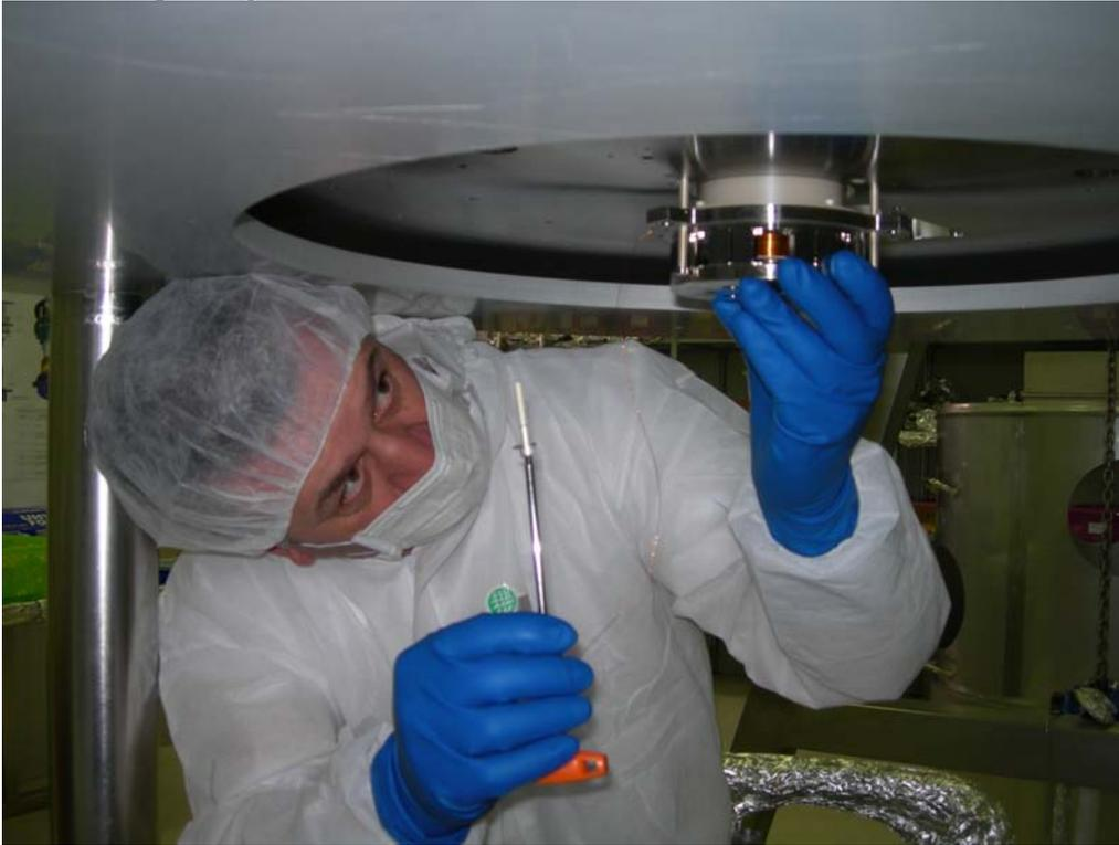
the three push and the three pull screws are used ...
