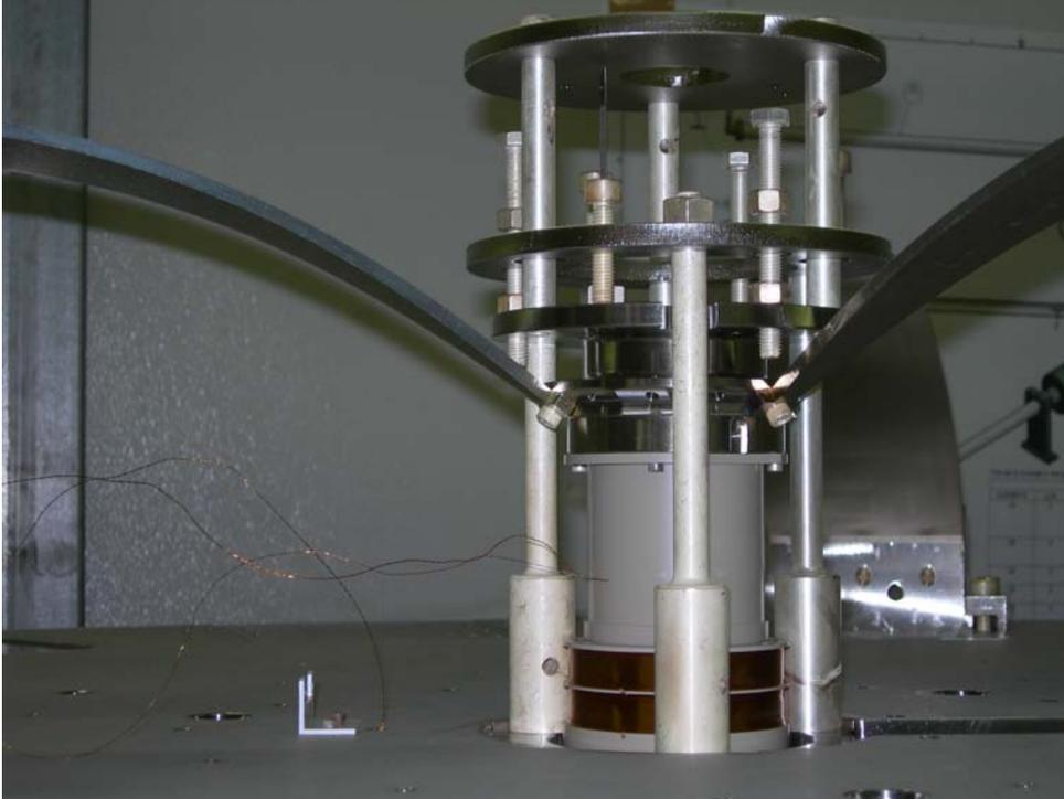
The push-pull screws are also used for the transversal centering of the secondary to the Keystone, which for the initial tuning is made with a PEEK wedge gauge, against the M12 load threaded rod.
