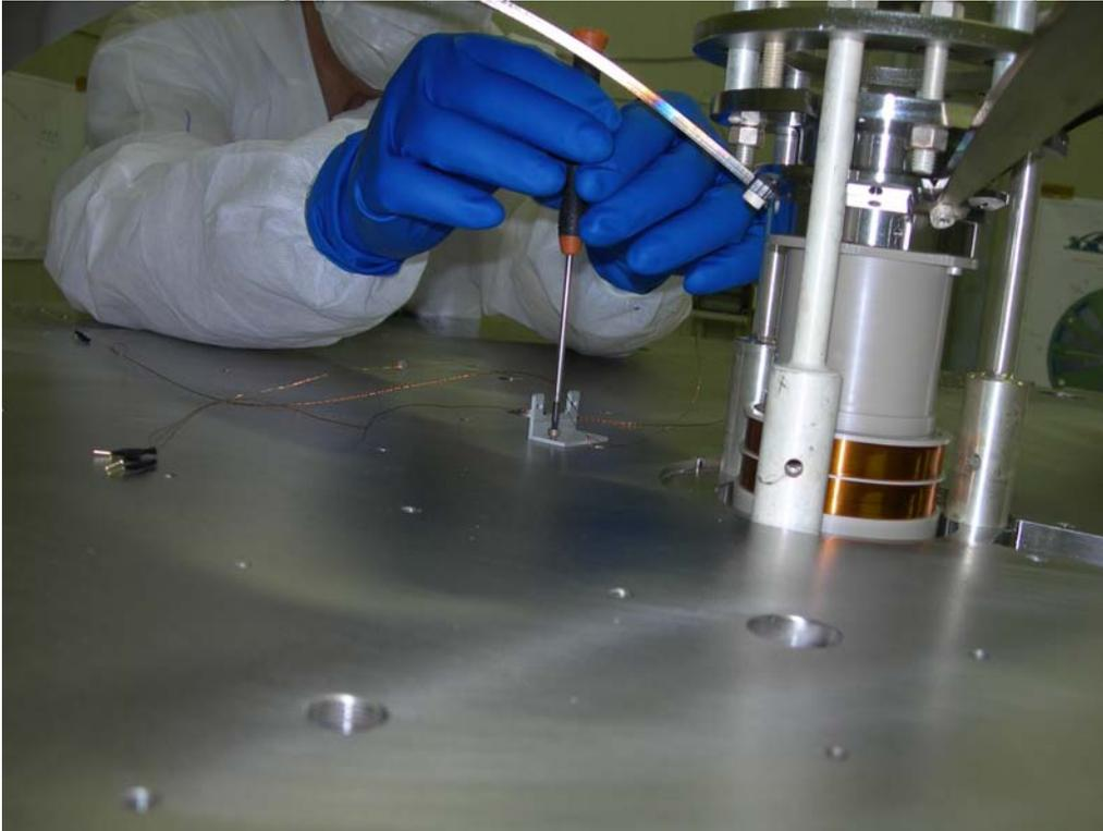
The cabling hexagon is mounted below the top filter
