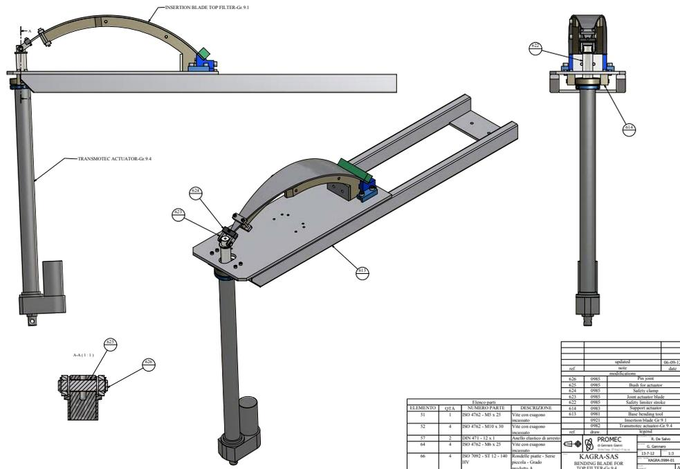
The photo shows the size of the actuator and of the blades. The drawing shows how the -pre-stress is held after the blade has been pulled, before it is mounted on the filter. Please also see the related movie in JGW-G1301580. <http://gwdoc.icrr.u-tokyo.ac.jp/cgi-bin/DocDB/ShowDocument?docid=1580>
