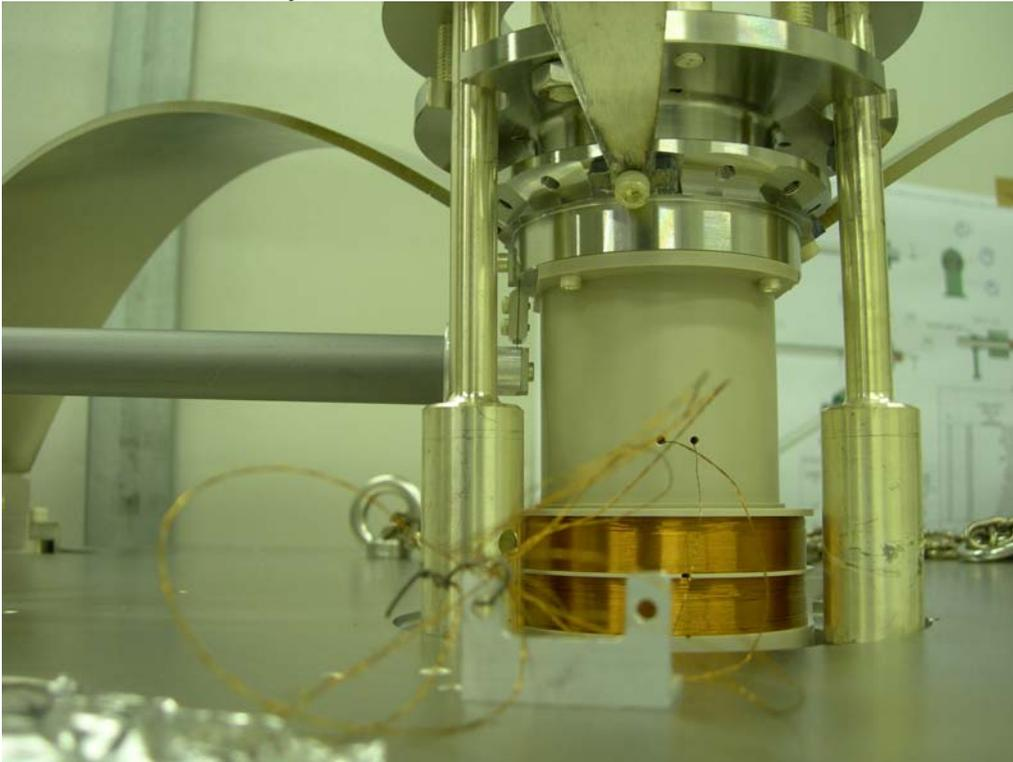
The magic wand is ready. The pre-isolator filter is ready for shipment, with the exception of the magnetic dampers and rotational mechanism, which are packed separately.
