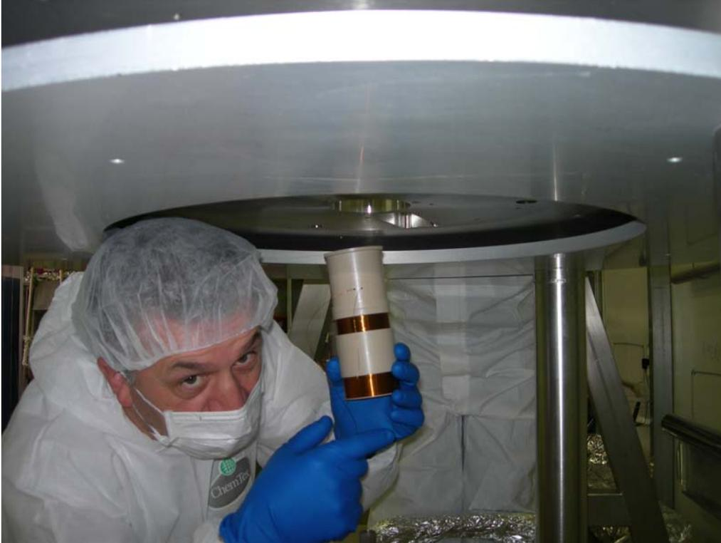
A second operator holds the coil and orients the wiring towards the connector stand
