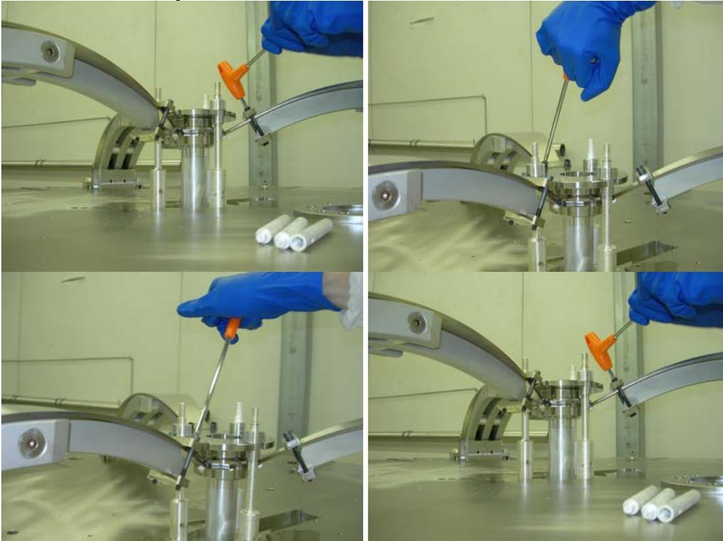
Then the pre-stressing arcs are released from the blade bases and removed.
