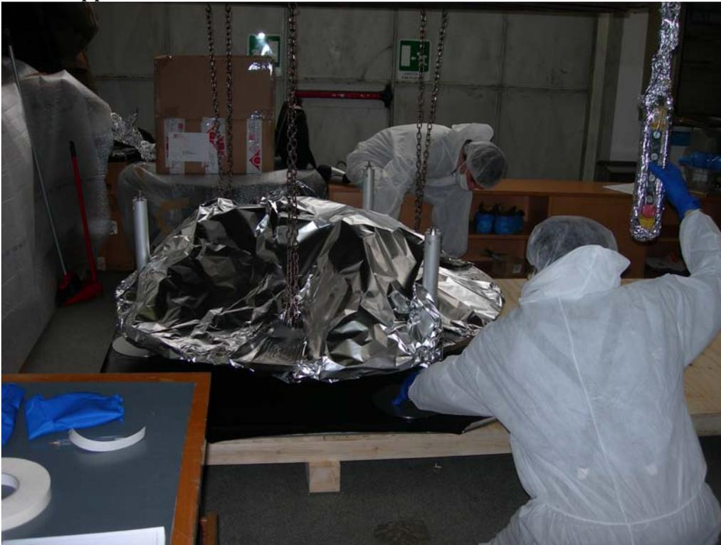
After tightly bolting the feet on the base the first filter is ready for shipment
