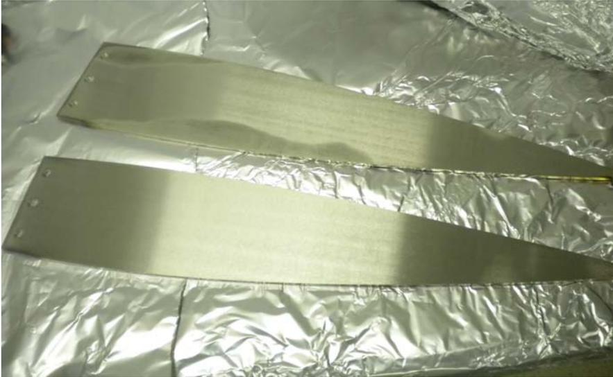
The thickness of all blades was checked with a Palmer micrometer and, more precisely, with an electronic scale with 1 g error over 2100 g weight. The mass is proportional to the average thickness, therefore a better indicator of the blade's strength as a spring. A mass fluctuation of only 0.1% between blades was measured.
