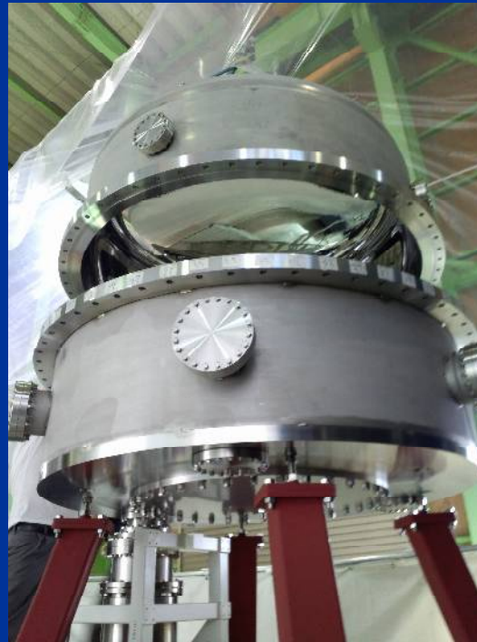
Seal test of the top-chamber
