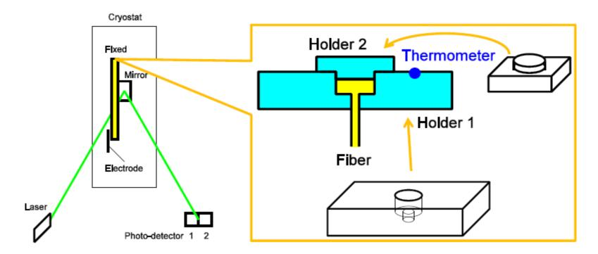
Mechanical loss measurement of Sapphire fibers/disks.
