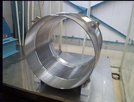
Bellows for each duct
