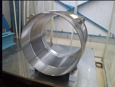
Bellows for each duct
