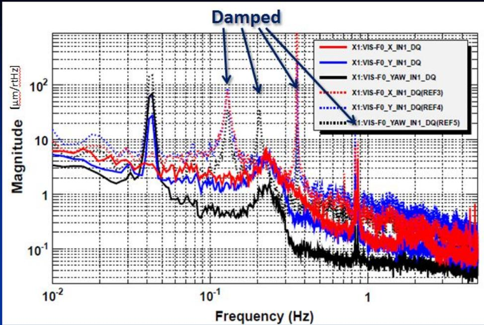
Control test of the inverted pendulum. Some resonances were damped effectively.
