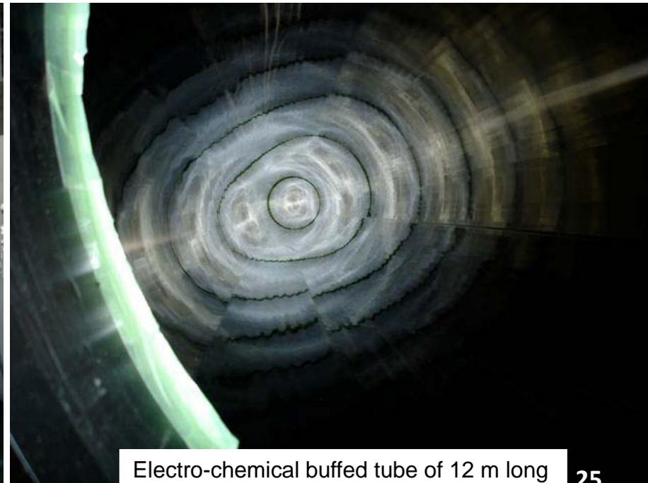
Electro-chemical buffed tube of 12 m long
