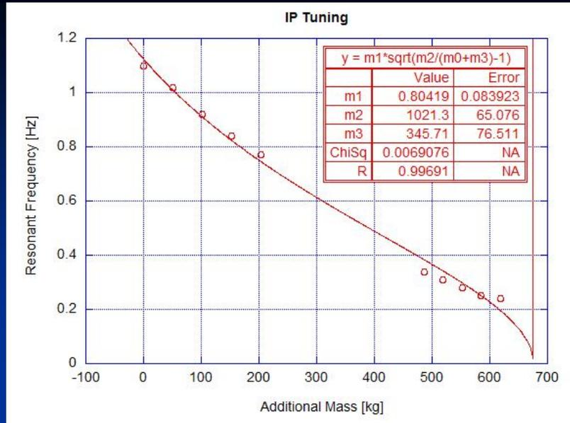
Tuning of the inverted pendulum. The present resonant frequency is 130mHz.
