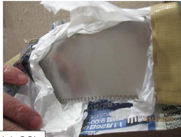
Laser cutting (1 mm thick SS)
