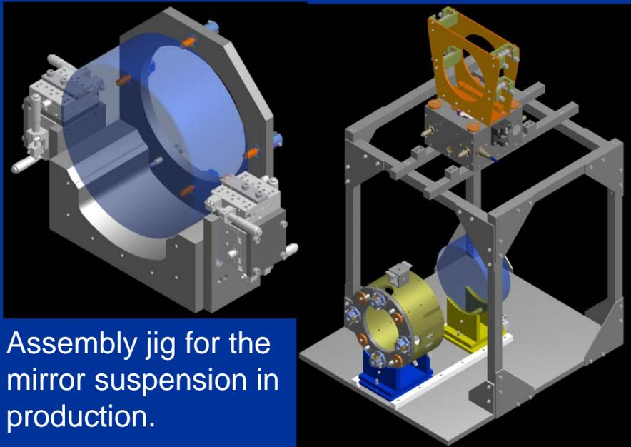
Assembly jig for the mirror suspension in production.
