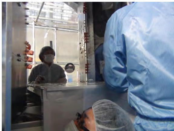
Al sphere for an initial cooling test of mirror suspension
