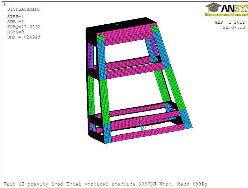
Fig.8 second mode, bending, for case 1 and 2
