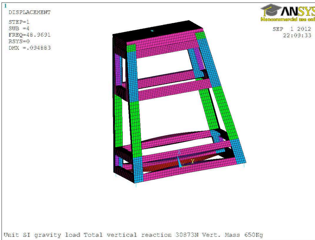
Fig.10 fourth mode, torsional, for case 1 and 2
