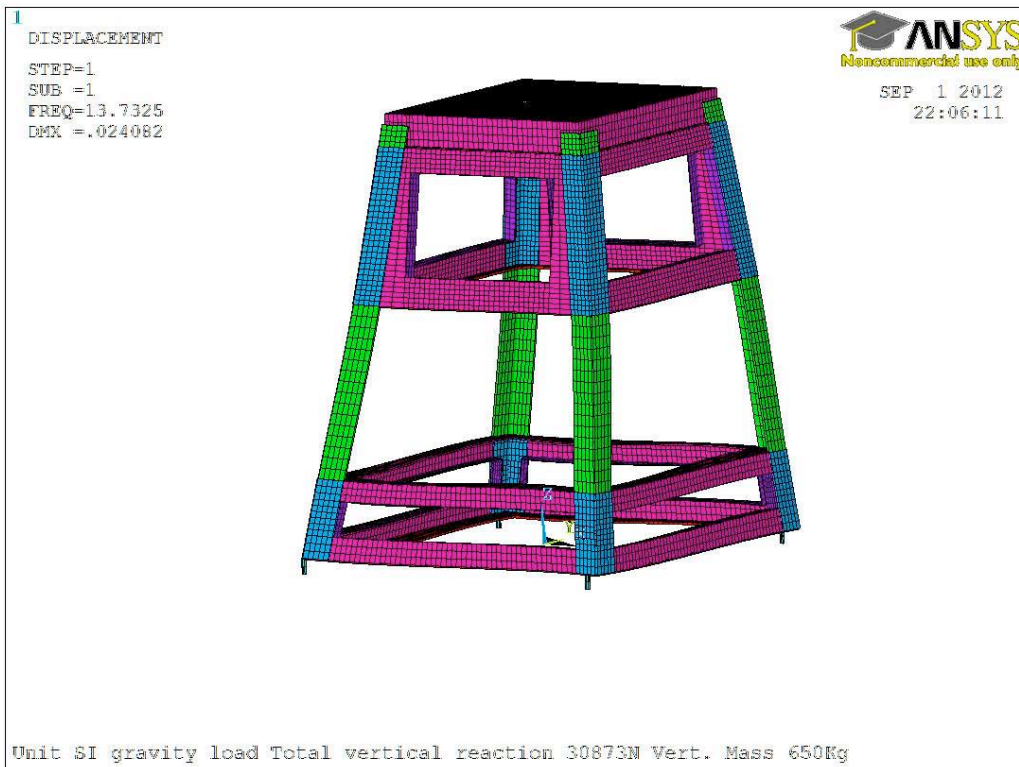
Fig.7 Fundamental mode, bending, for case 1 and 2
