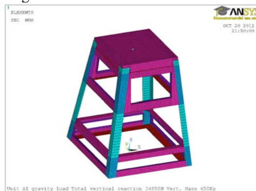
Fig. 2 Finite Element Analysis model
