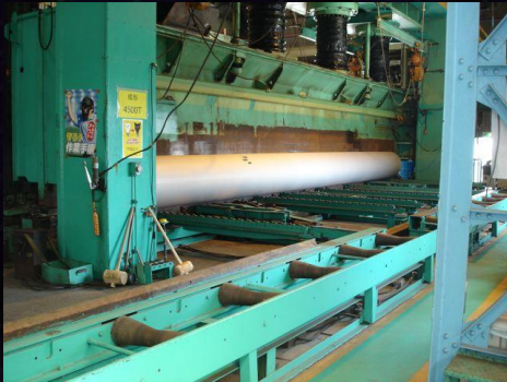
Press to form a duct
