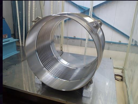
Bellows for each duct
