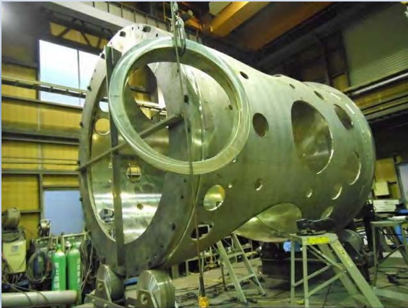
Main body ( \Phi 2.6\text{m} , H3.6m)
