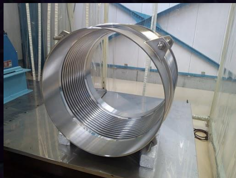
Bellows for each duct
