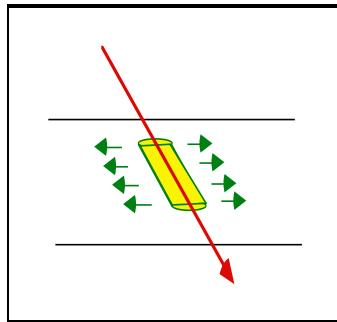
Interaction of a particle with a bar: ionization energy lost is converted in thermal heating and therefore pressure wave. The detection mechanism is quite simple, no threshold in  $\beta$
