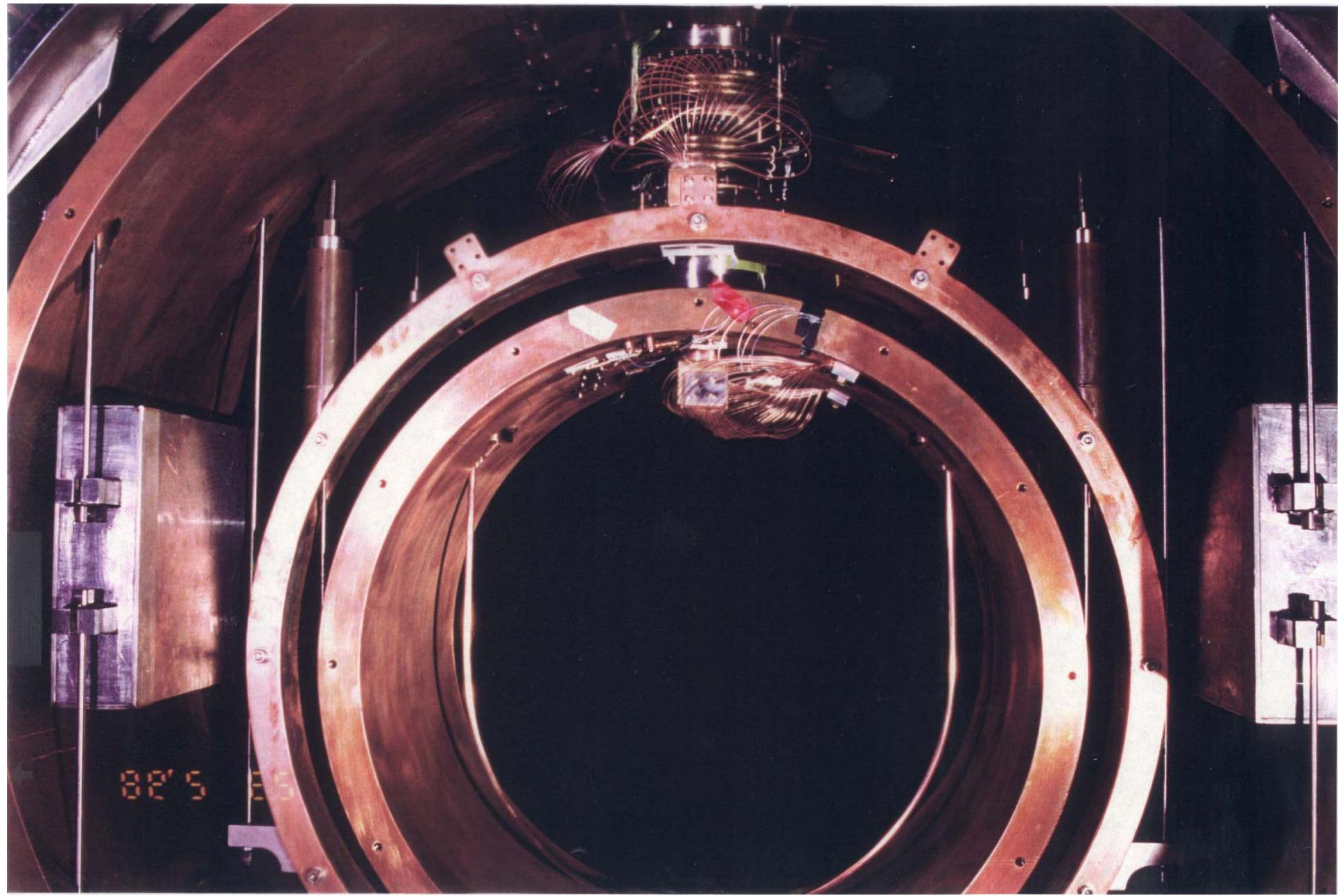
**Suspension and thermal link of an ultralow temperature GW antenna.**
