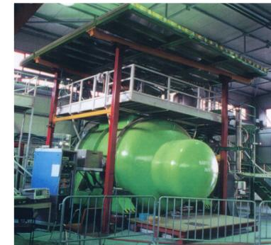
Nautilus is equipped with streamer tubes particle detectors
