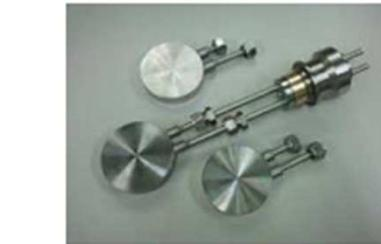
Three sets of exchangeable target holder, each holding two sputter targets
