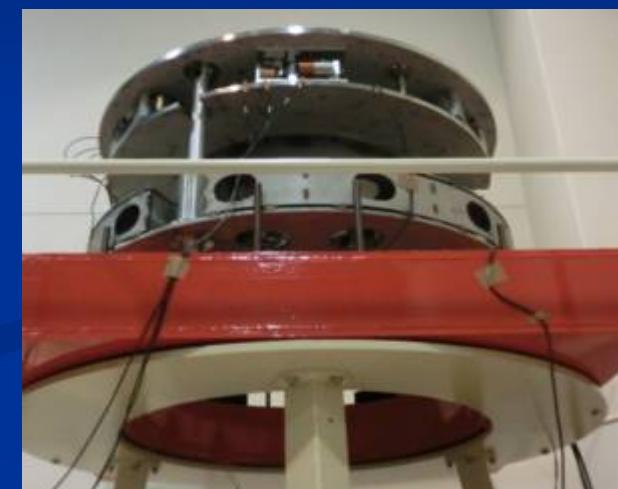
Motor sliders and LVDT-actuator modules were assembled onto the IP with cabling.
