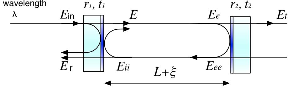
Figure 1: A Fabry-Pérot cavity and its relevant fields.
