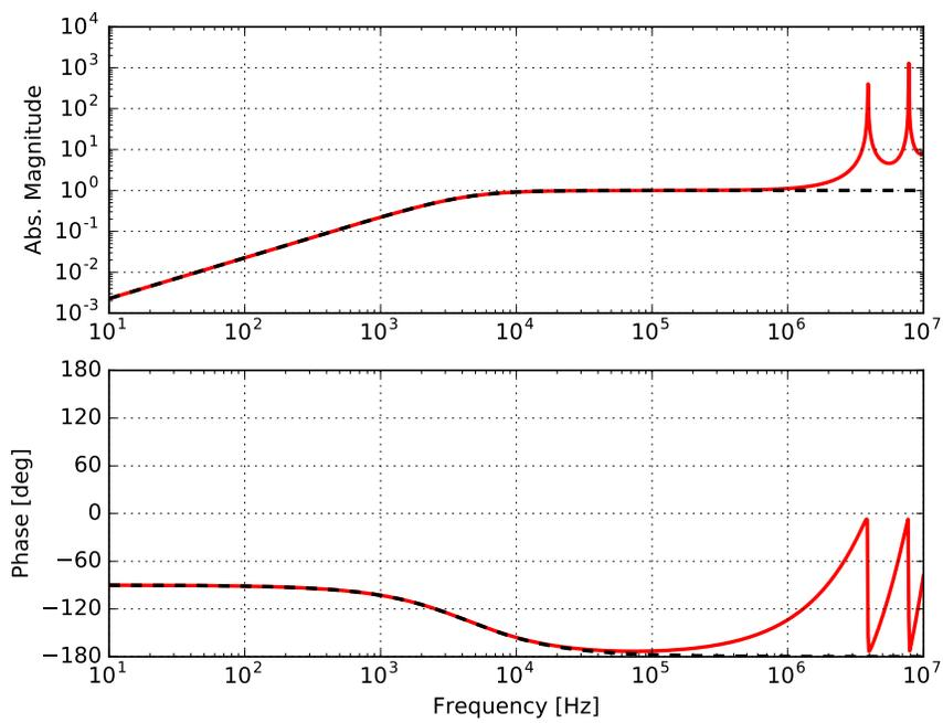
Figure 2: Bode plot of the transfer functions. The cavity pole is set to 4.4 kHz. The red curve is the one using the full expression (16) and the black dashed curve is from the approximated form (17).
