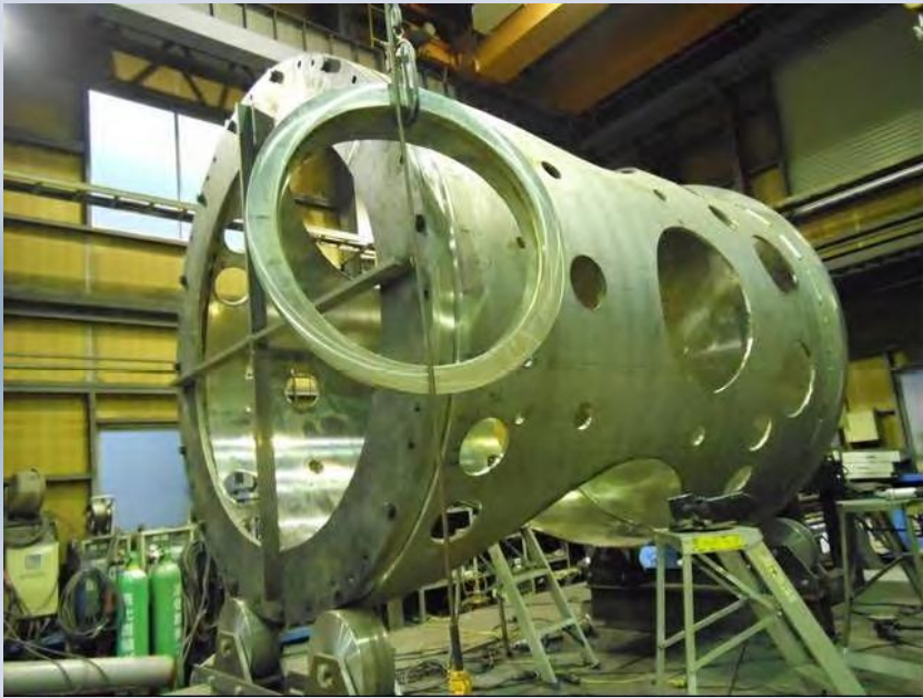
Main body ( \Phi 2.6\text{m} , H3.6m)
