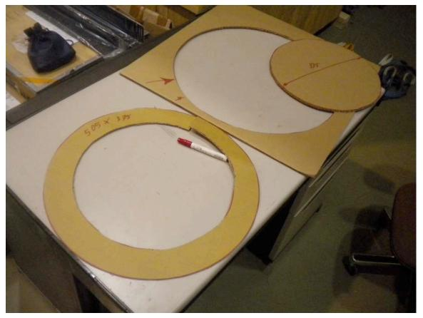
Then I lifted one edge and inserted it into the pipe, and obtained a nice spiral with a nice fit. Despite the crude model, I obtained a pitch not far from the calculated 537 mm.
