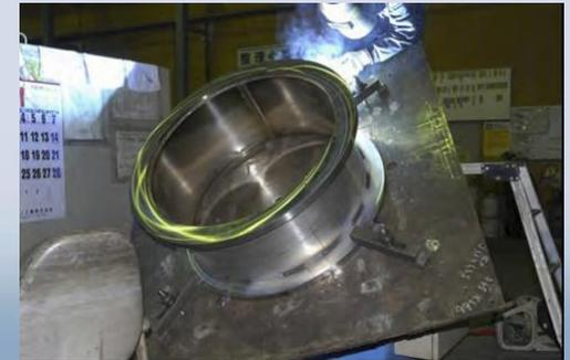
Connection port to cryo-cooler unit
