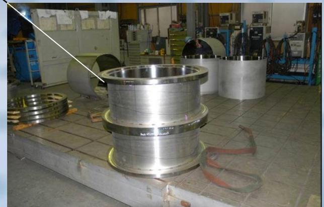
Connection port to cryocooler unit
