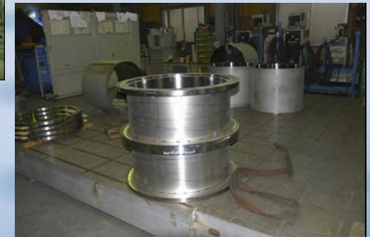
Connection port to cryo-cooler unit
