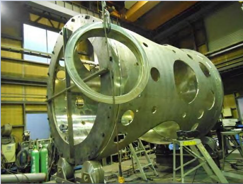
Main body ( \Phi 2.4\text{m} , H3.8m)
