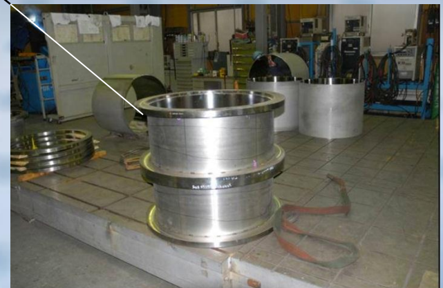
Connection port to cryocooler unit
