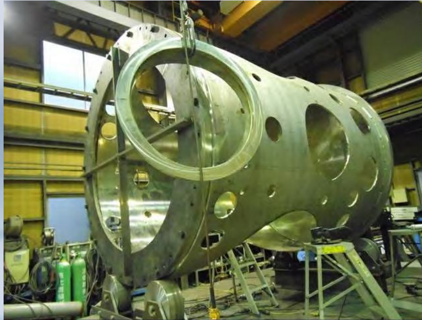
Main body ( \Phi 2.4\text{m} , H3.8m)
