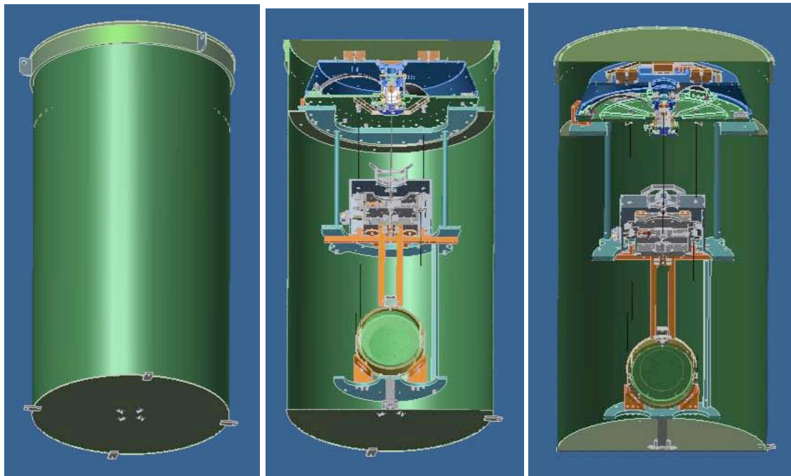
Figure 16: The transport tank for the payload is much smaller. The bottom plate of the tank is provided with bolting lips to attach the tank to a transport pallet. The payload locked into its safety structure is bolted from above onto a circular shelf.
