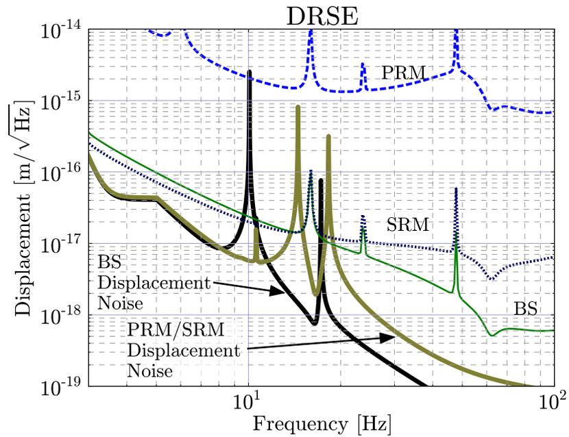
Figure 4.2: Displacement noise requirements for auxiliary mirrors: DRSE
