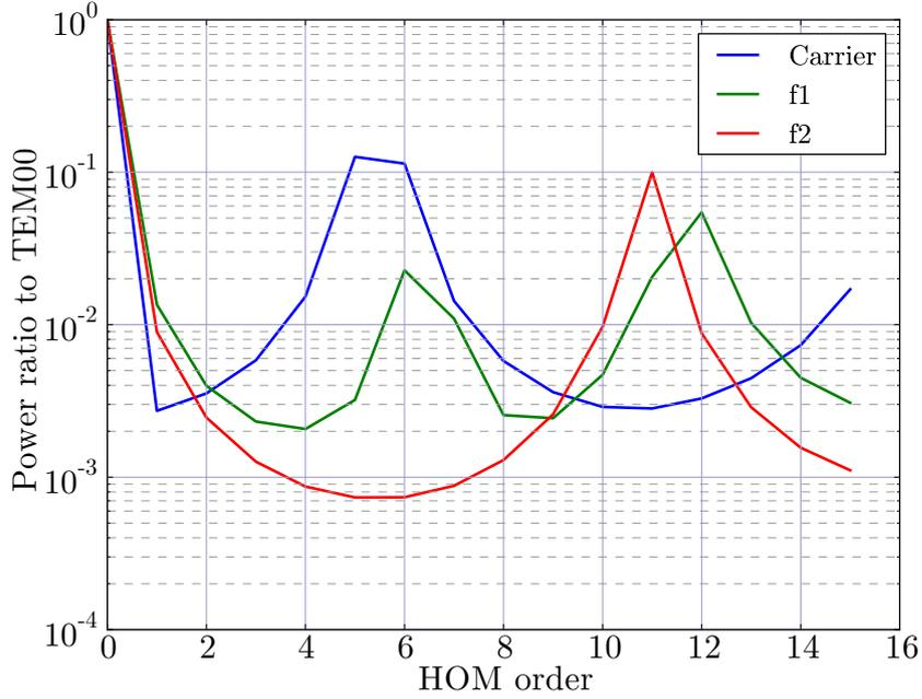
Figure 2.17: HOM power ratio in the PRC: BRSE.
