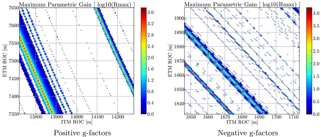
Figure 2.15: Maps of the maximum parametric gain as functions of the ROCs of the test masses. Left: positive g-factor, Right: negative g-factor. The ROCs are swept by  $\pm 2\%$  of their nominal values. White areas correspond to  $R_{\max} < 1$ .
