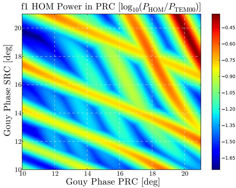
Figure 2.19: The maximum HOM power ratio of the f1 SB in the PRC: BRSE.
