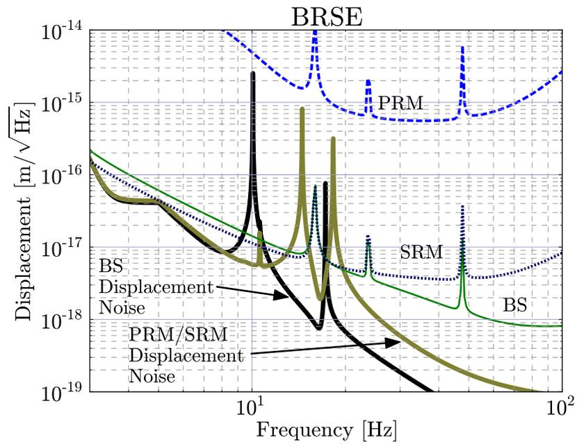
Figure 4.1: Displacement noise requirements for auxiliary mirrors: BRSE
