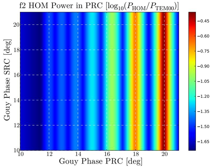
Figure 2.20: The maximum HOM power ratio of the f2 SB in the PRC: BRSE.
