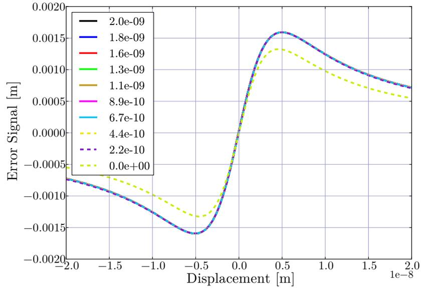
Figure 6.3: THD PRCL error signal with various CARM offset. Signal port is REFL, demodulated at  $3 \times f_2$  in I-phase.
