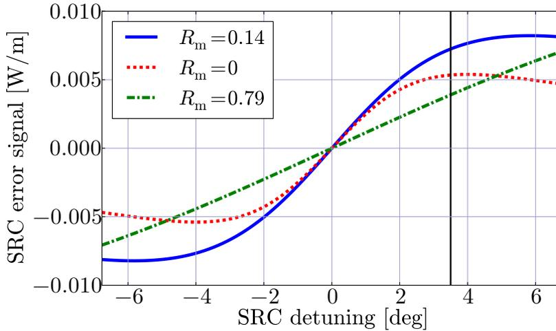
Figure 2.16: SRCL error signals for three different values of  $R_m$ . The horizontal axis is the detuning of the SRC in terms of the one-way phase shift. The vertical axis is the signal from the POP port demodulated at the f1 frequency. The vertical line shows the operation point of DRSE ( $3.5^\circ$ ).
