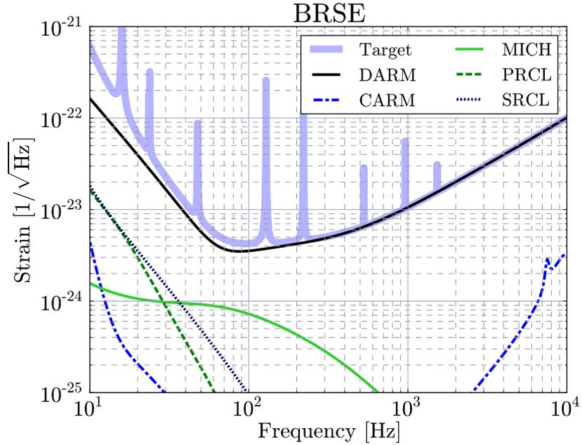
Figure 3.5: Loop Noise Coupling with Feed Forward: BRSE
