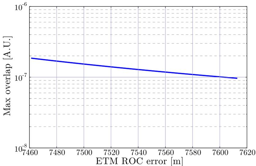
Figure 2.14: Figure of merit of the overlap between the RF SB harmonics and the HOMs when the ETM ROC is swept.  $g$ -factor is positive.
