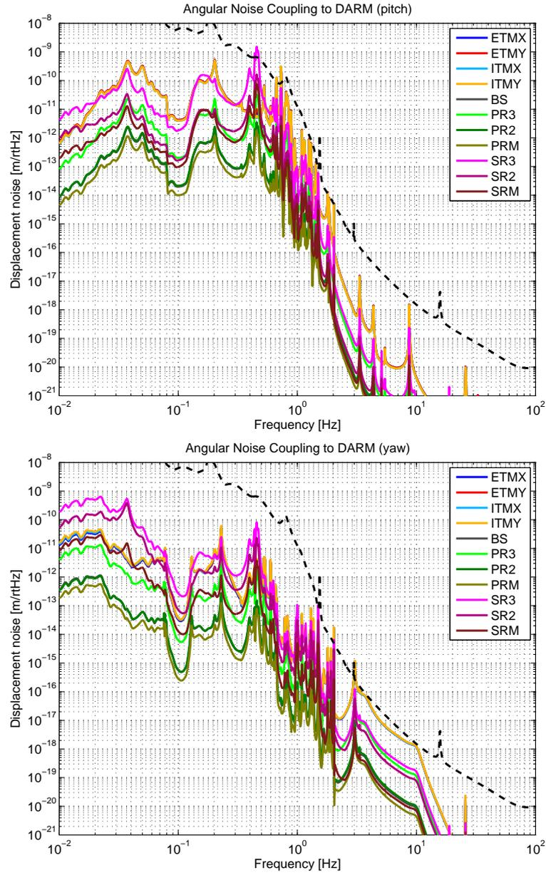
Figure 5.4: Angular noise coupling to DARM (top: pitch, lower: yaw). The dotted line shows bKAGRA design sensitivity.
