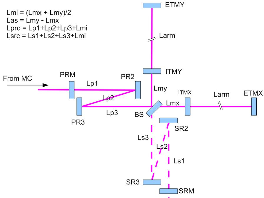
Figure 2.1: Schematic of the main interferometer and the naming convention of IFO parameters
