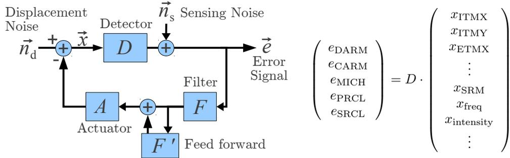
Figure 3.2: Block diagram of the feedback loops. The real DOF vector  $\vec{x}$  contains the displacement of each mirror and other dynamic degrees of freedom in the interferometer, such as laser frequency and intensity. It is converted to the vector  $\vec{e}$  of the error signals in the canonical DOFs by the detector matrix  $D$ . All the matrices in the figure are frequency dependent.
