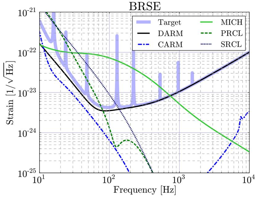
Figure 3.3: Loop Noise Coupling: BRSE
