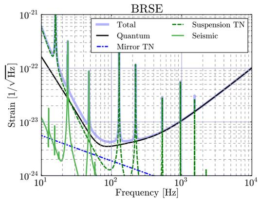
Figure 1.1: bKAGRA Target Sensitivity in the BRSE mode
