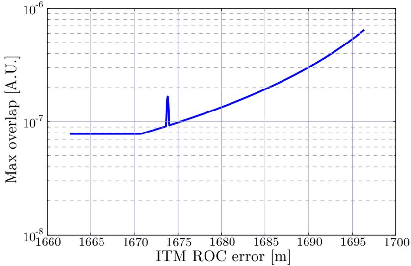
Figure 2.11: Figure of merit of the overlap between the RF SB harmonics and the HOMs when the ITM ROC is swept.  $g$ -factor is negative.
