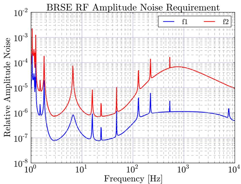
Figure 4.12: RF oscillator amplitude noise requirements: BRSE
