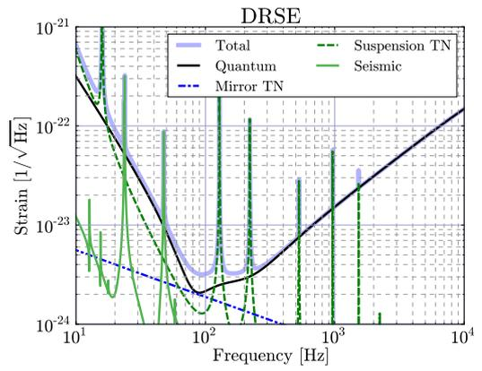
Figure 1.2: bKAGRA Target Sensitivity in the DRSE mode
