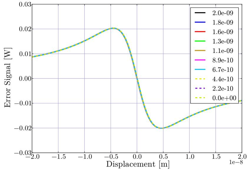
Figure 6.6: NRS PRCL error signal with various CARM offset. Signal port is REFL, demodulated at  $|f_3 - f_2|$  in I-phase.
