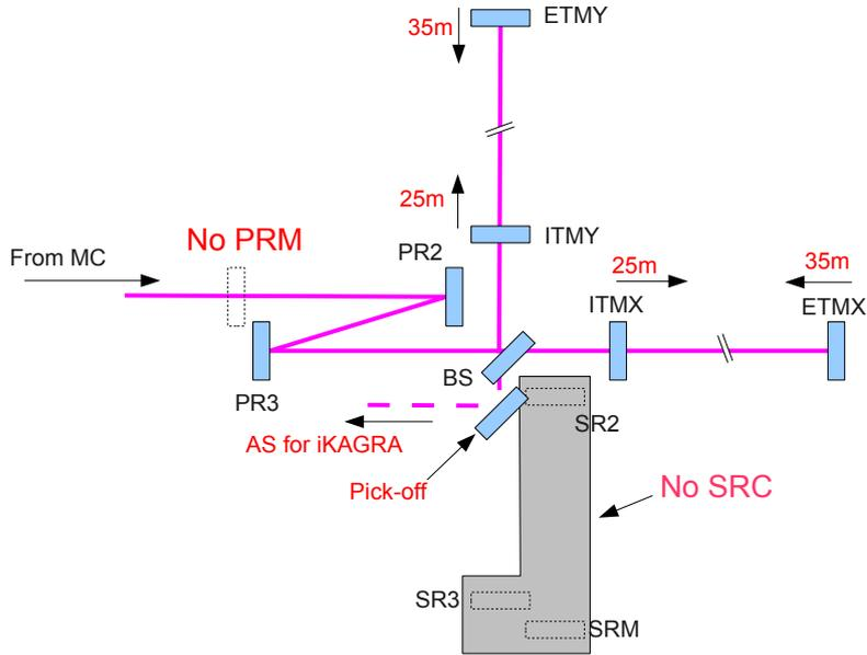
Figure 9.1: Differences between the iKAGRA and bKAGRA optical configurations/layouts.
