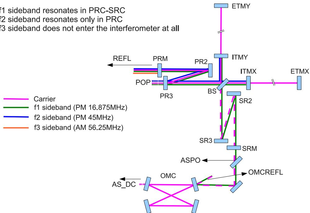
Figure 3.1: RF sideband resonant conditions and signal ports. POP is drawn at the transmission of PR3 to avoid congestion of the diagram. However, POP is actually planned to be picked up from the back of PR2 because the beam size is much smaller there.
