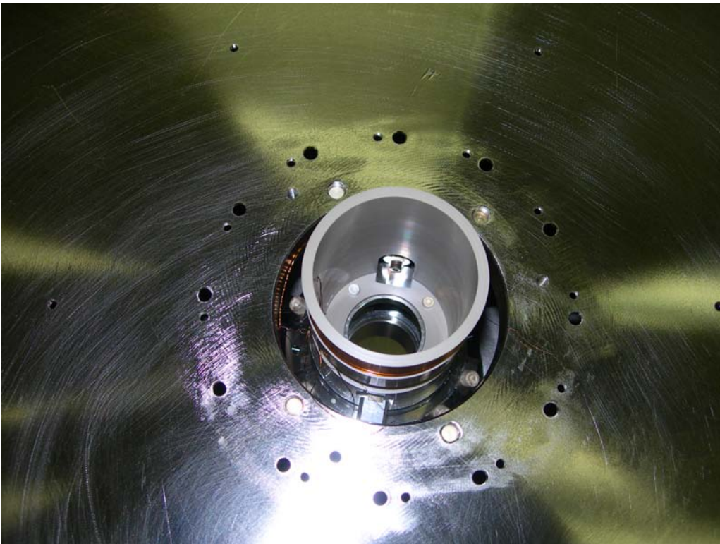
After mounting the magic wands, the LVDT primary and the actuation coil are mounted on the filter.
