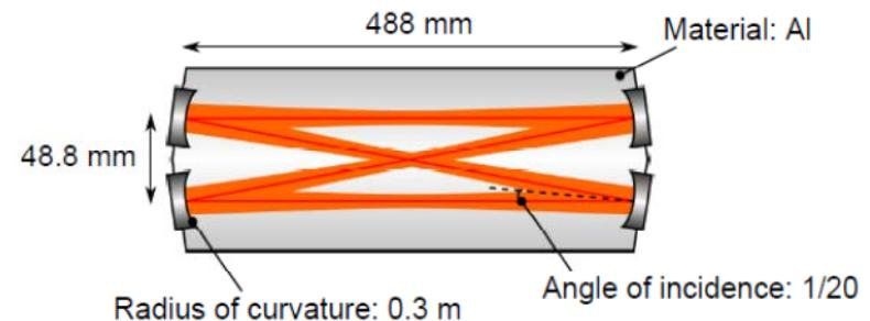
This cavity is put in air tight case, not in vacuum.
