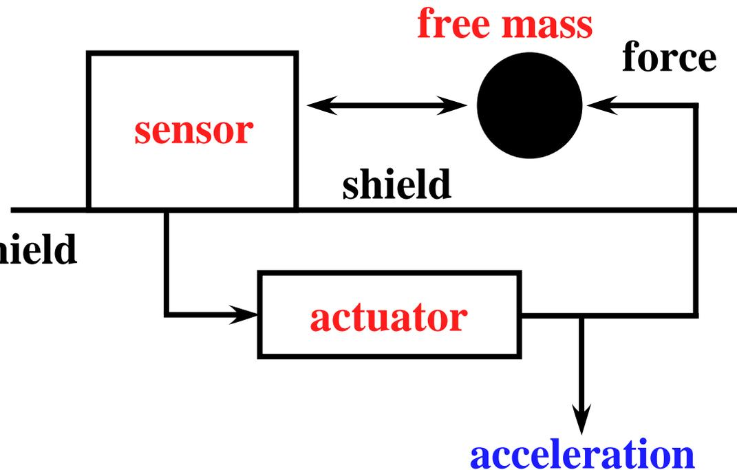
→ **Acceleration** of shield is derived from **feedback signal**.
